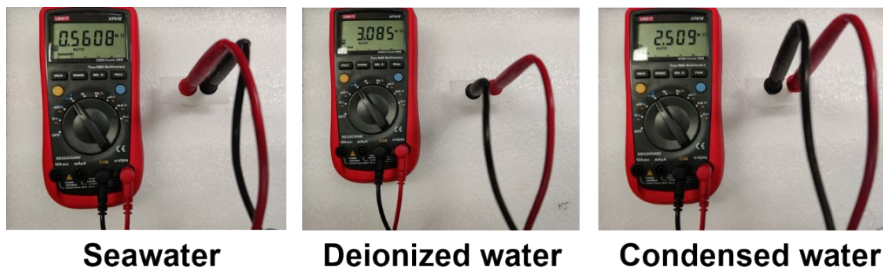
Fig. S20 Digital photographs for the resistance value comparison of seawater, deionized water and condensed water.
