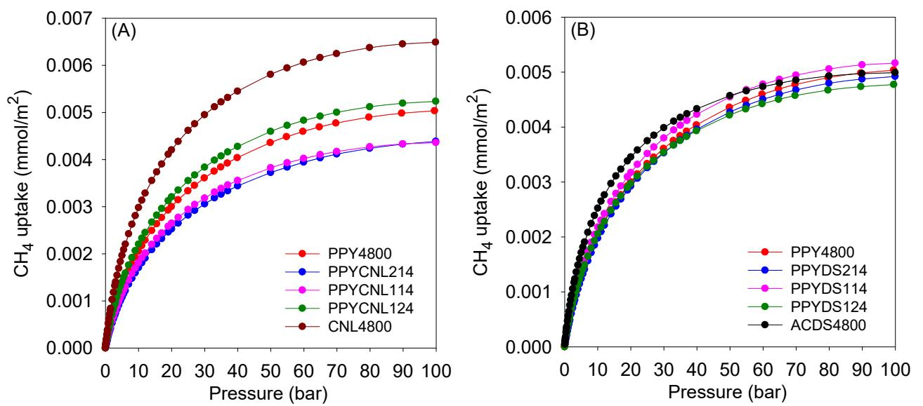
Figure S6. Excess gravimetric methane uptake density of activated carbons derived from single precursor, PPY4800 (polypyrrole, PPY), CNL4800 (CNL carbon) and ACDS4800 (ACDS carbon) and from pre-mixed precursors containing PPY and (A) CNL carbon or (B) ACDS carbon at various weight ratios.
