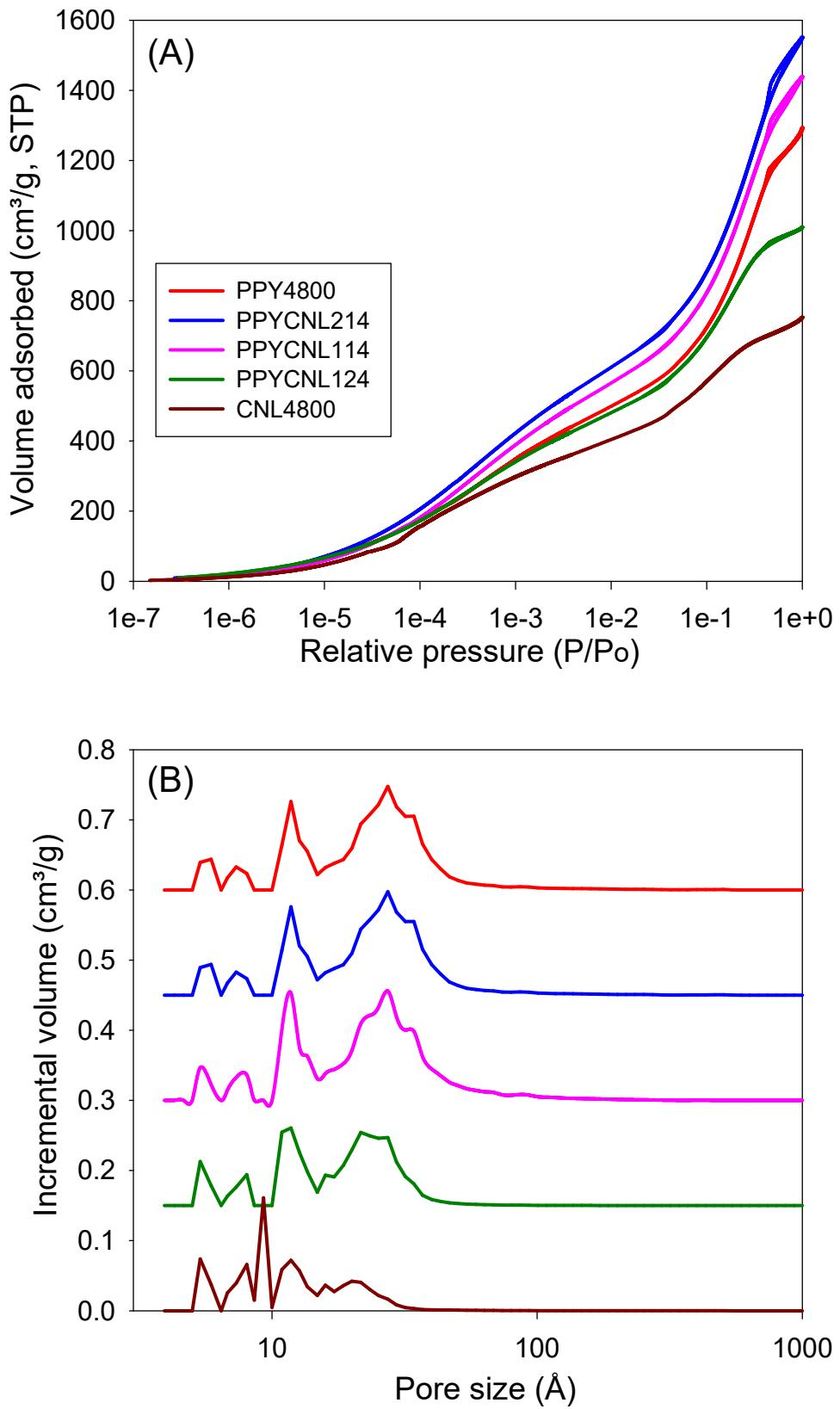
Figure S5A. Semi-log plots of (A) Nitrogen sorption isotherms and (B) pore size distribution curves of activated carbons derived from single precursor, PPY4800 (polypyrrole, PPY) and CNL4800 (CNL carbon) and from pre-mixed precursors containing PPY and CNL carbon at various weight ratios.
