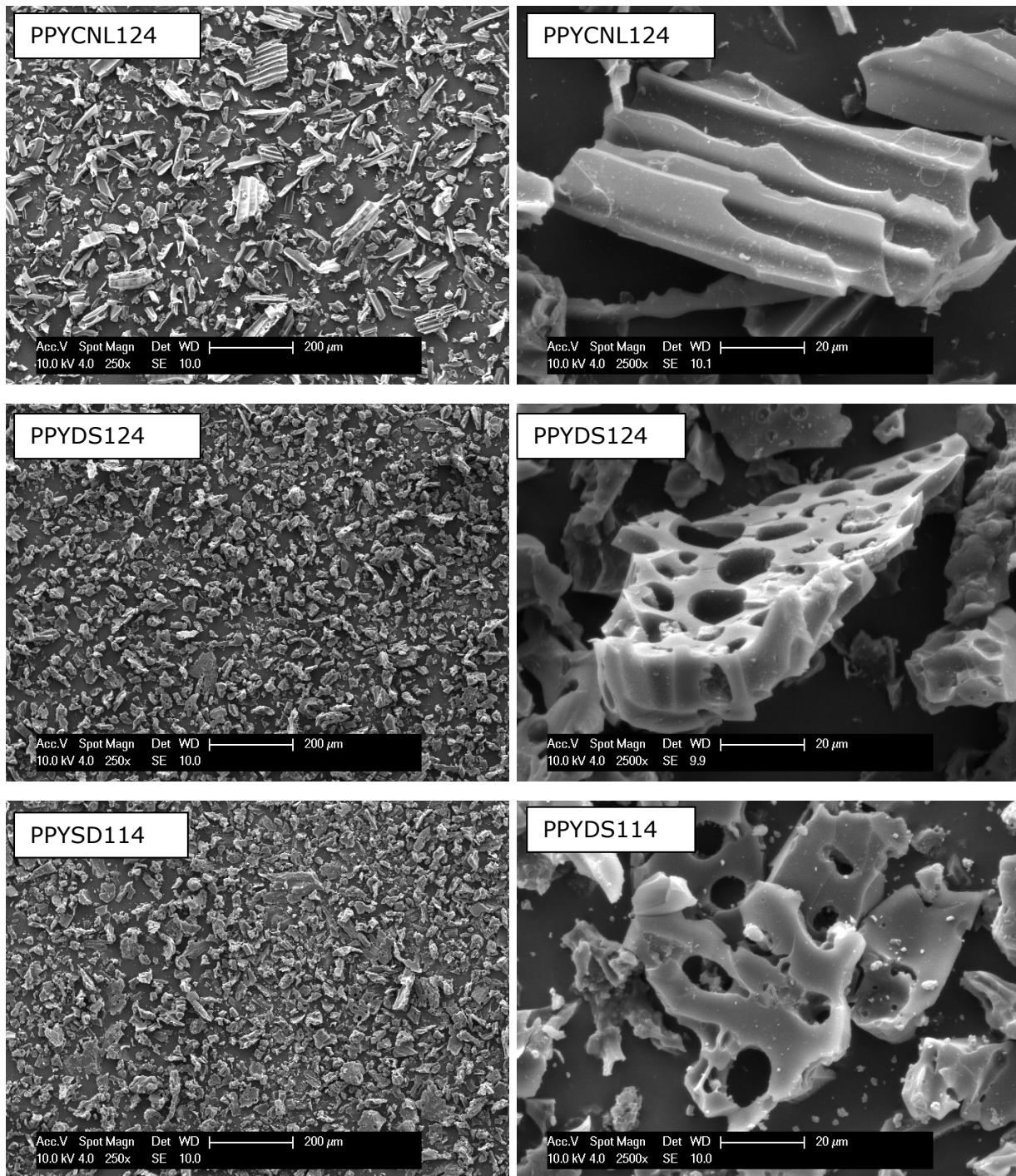
Figure S3. Representative SEM images of activated carbons derived from pre-mixed precursors.
