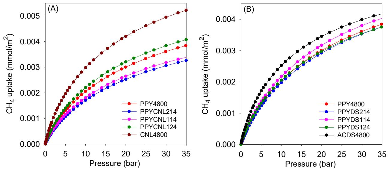
Figure S7. Excess gravimetric methane uptake density at low pressure (0 – 35 bar) of activated carbons derived from single precursor, PPY4800 (polypyrrole, PPY), CNL4800 (CNL carbon) and ACDS4800 (ACDS carbon) and from pre-mixed precursors containing PPY and (A) CNL carbon or (B) ACDS carbon at various weight ratios.
