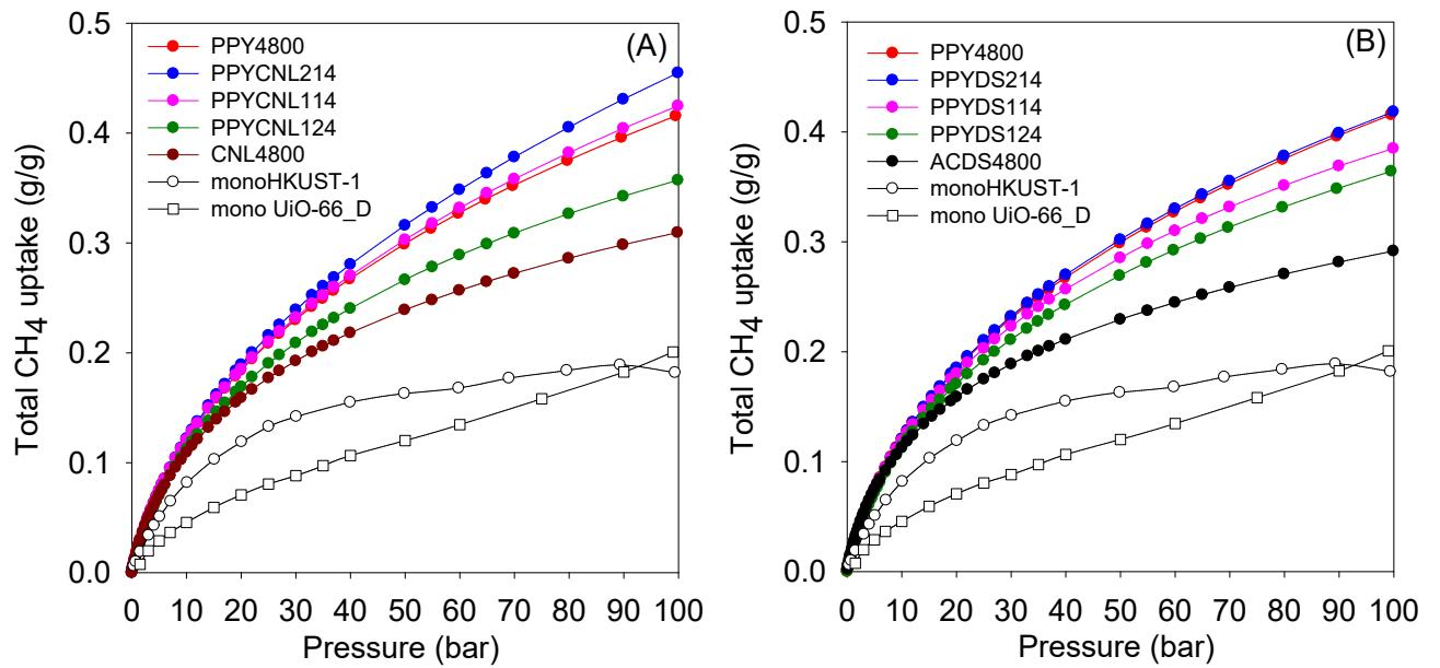
Figure S10. Total gravimetric methane uptake (gCH<sub>4</sub> g<sup>-1</sup>) of activated carbons derived from single precursors (PPY4800, CNL4800, ACDS4800) or (A) PPY/CNL pre-mixtures or (B) PPY/DS pre-mixtures compared to storage capacity of monolithic <sub>mono</sub>HKUST-1 and <sub>mono</sub>UiO-66\_D.
