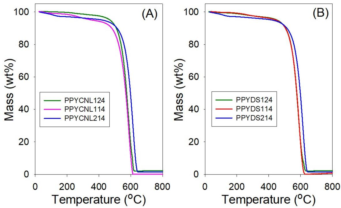
Figure S1. Thermogravimetric analysis (TGA) curves of activated carbons derived from pre-mixed mixtures of polypyrrole (PPY) and (A) CNL carbon or (B) ACDS carbon.
