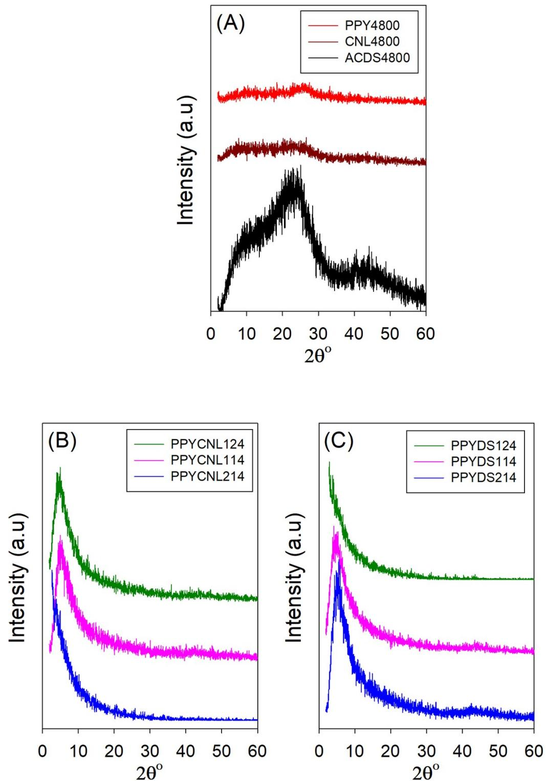
Figure S2. Powder XRD pattern of (A) Polypyrrole, CNL carbon and ACDS carbon precursor materials, and (bottom panels) of activated carbons derived from pre-mixed mixtures of polypyrrole (PPY) and (B) CNL carbon or (C) ACDS carbon.
