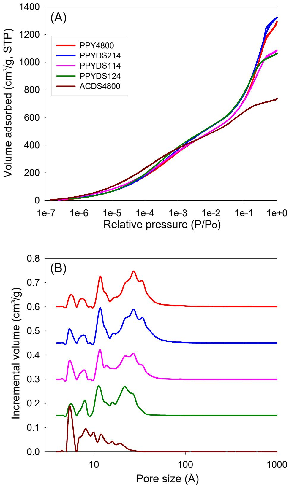
Figure S5B. Semi-log plots of (A) Nitrogen sorption isotherms and (B) pore size distribution curves of activated carbons derived from single precursor, PPY4800 (polypyrrole, PPY) and ACDS4800 (ACDS carbon) and from pre-mixed precursors containing PPY and ACDS carbon at various weight ratios.
