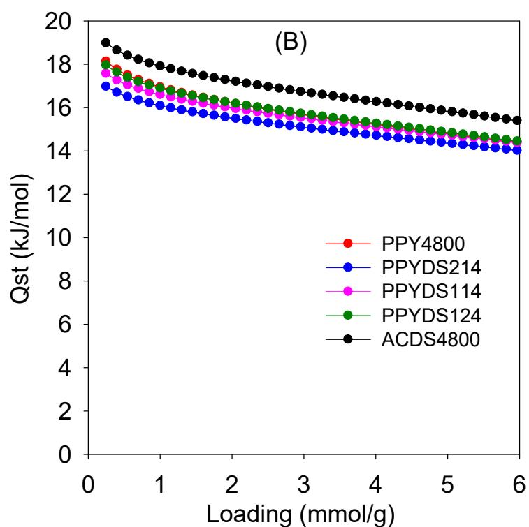
Figure S8. Isosteric heat of adsorption ( $Q_{st}$ ) as a function of methane loading of activated carbons derived from single precursor, PPY4800 (polypyrrole, PPY), CNL4800 (CNL carbon) and ACDS4800 (ACDS carbon) and from pre-mixed precursors containing PPY and (A) CNL carbon or (B) ACDS carbon at various weight ratios.
