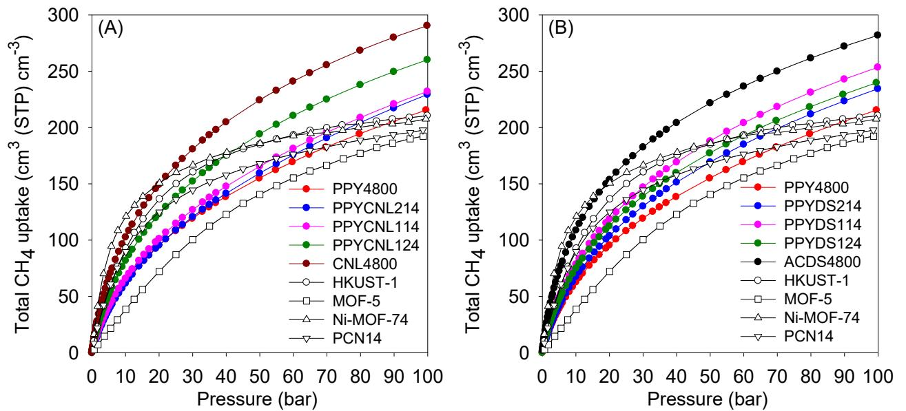
Figure S9. Total volumetric methane uptake of activated carbons derived from single precursors (PPY4800, CNL4800, ACDS4800) or (A) PPY/CNL or (B) PPY/DS pre-mixtures compared to benchmark MOF materials. The uptake of MOFs, allows for a 25% reduction of values calculated using crystallographic density.
