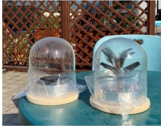
Fig S33. The photograph of device for the “sorption tree” and the “sorption plane” during the desorption process under the sunlight.
