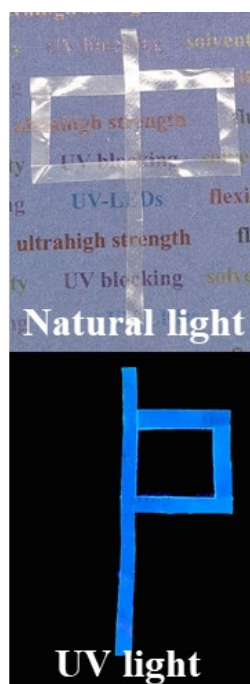
Figure S17. Fluorescent anti-counterfeiting of films under UV irradiation (365 nm)
