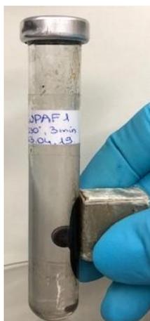
**Fig. S51** Photos demonstrating the ferromagnetism of the Pd/Fe<sub>3</sub>O<sub>4</sub>-on-ZIF8-NP after washing in the MW-tube via the action of the magnet (the black layer near the cube-shaped magnet is the sample with the magnetic stirring bar on top of it). The photo is taken on a sample under inert atmosphere, but the ferromagnetism is retained in the air for days at least (seemingly indefinite time).
