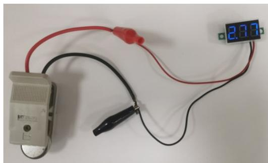
**Fig. S18.** Digital photograph of LED illuminated by Li-S battery based on the BP@FeCoO electrode.
