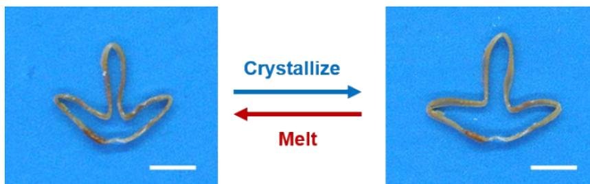
**Figure S11.** The reversible actuation of the welded “bird paw” sample (scale bar is 1 cm).
