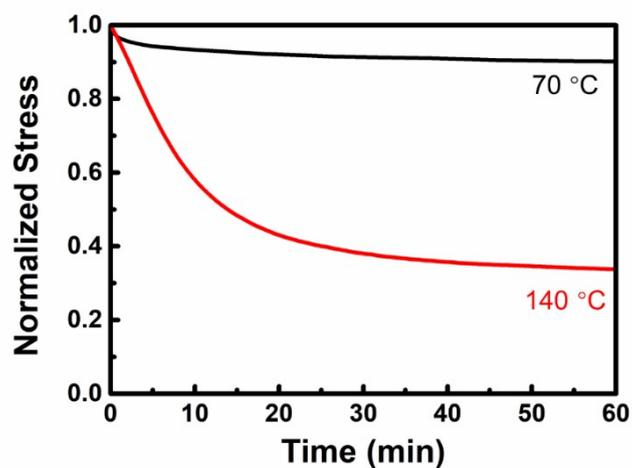
**Figure S6.** Typical stress relaxation curves of the sample at 70 °C and 140 °C.
