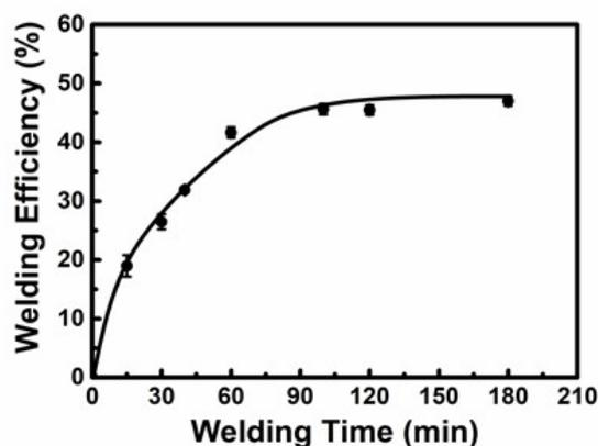
**Figure S10.** The welding efficiency of the sample with 70% BA. The welding efficiency is calculated by dividing the strain at break of the welded sample by the original sample.
