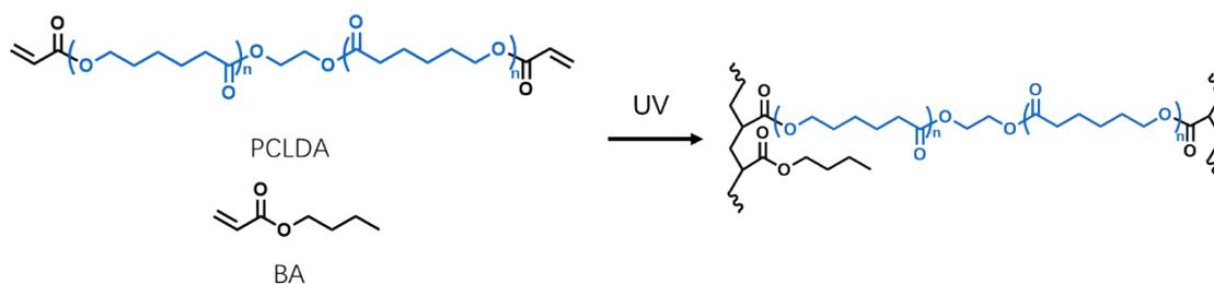
**Figure S2.** Synthetic scheme for the converse two-way SMP.
