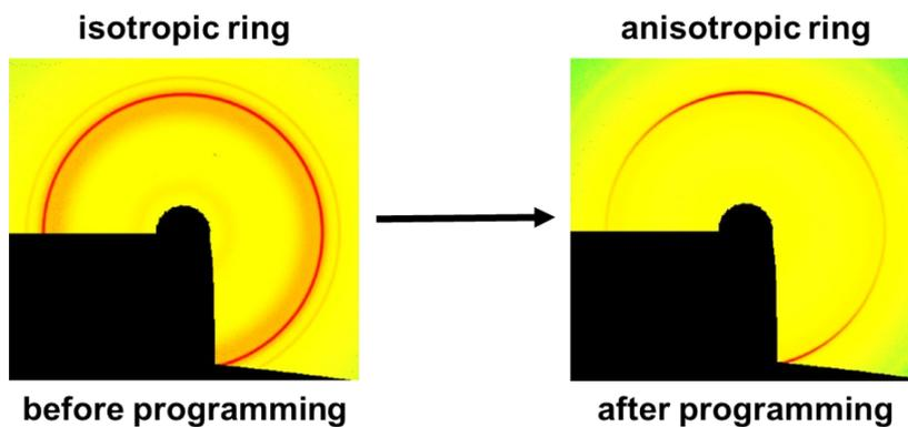
**Figure S4.** The 2D-WXRD figures of the sample before and after programming. The anisotropic ring after programming is contrary to the conventional result (reference 1) that the orientation is parallel to the programming, proving the perpendicular orientation.
