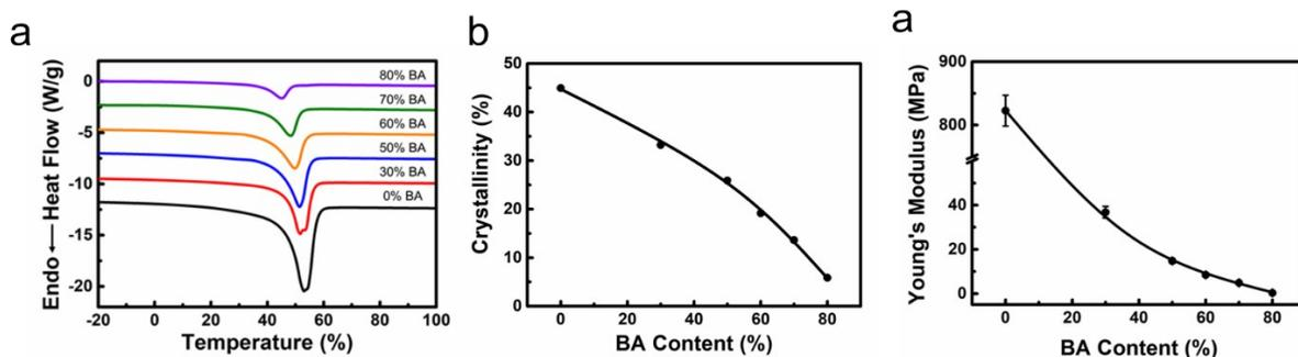
**Figure S7.** Thermal analysis and modulus of the samples with different BA contents. a) The DSC curves; b) The corresponding crystallinity; c) Young's modulus. The crystallinity is calculated as  $X_c = H_m/H_0$ , the  $H_m$  is the melting enthalpy,  $H_0$  is the ideal melting enthalpy of PCL.
