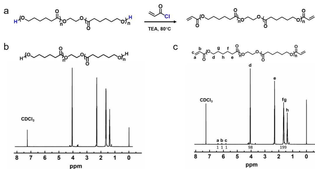
**Figure S1.** Synthesis of PCL diacrylate. a) Synthetic scheme for PCL diacrylate. b) <sup>1</sup>H-NMR spectrum of PCL. c) <sup>1</sup>H-NMR spectrum of the synthesized PCL diacrylate.
