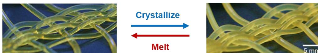
**Figure S9.** The reversible actuation of multi-strand fibers.
