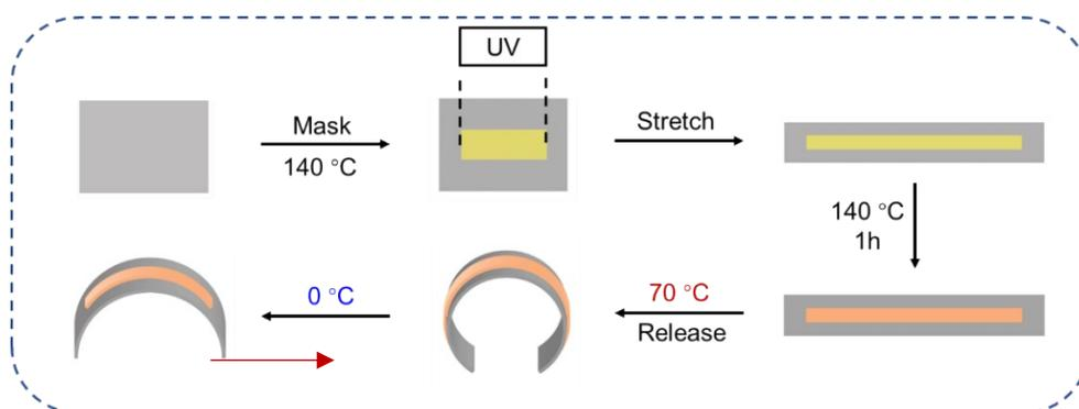
**Figure S13.** Schematic illustration of spatio-temporal programming reversible actuation by UV irradiation. (reversible actuation)
