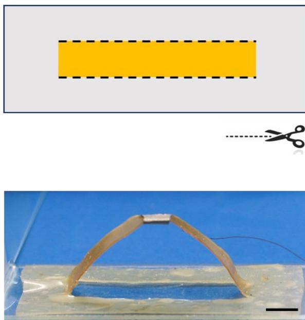
**Figure S14.** The photo-pattern 2D pattern with the strategic cutting and the corresponding thermosensitive switch after programming (scale bar is 1 cm)
