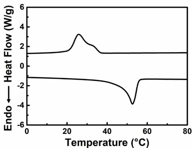
**Figure S5.** DSC curve of the sample with 70% BA.
