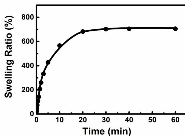
**Figure S12.** Swelling kinetics of the sample with 70% BA in photo-latent catalyst solution (mass ratio).
