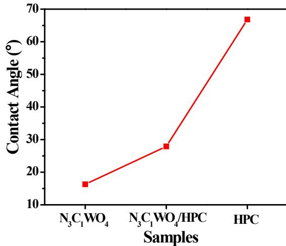
**Fig.S5.** The contact angles of the  $\text{Ni}_3\text{Co}_1\text{W}$ ,  $\text{Ni}_3\text{Co}_1\text{W}/\text{HPC}$  and HPC.
