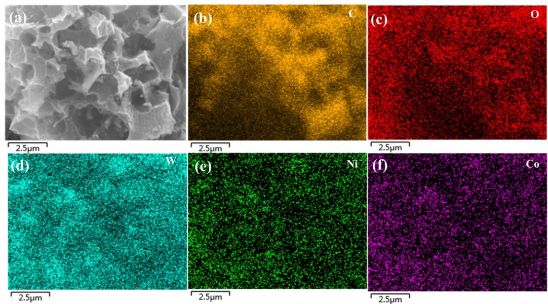
**Fig. S2.** (a) SEM images of the  $\text{Ni}_3\text{Co}_1\text{WO}_4/\text{HPC}$ , (b-f) EDS spectrum of  $\text{Ni}_3\text{Co}_1\text{WO}_4/\text{HPC}$  nanocomposite.
