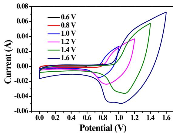
**Fig.S9.** CV curves of  $\text{Ni}_3\text{Co}_1\text{W}/\text{HPC}$  nanocomposite in different potential windows in a two-electrode system in 6M KOH.
