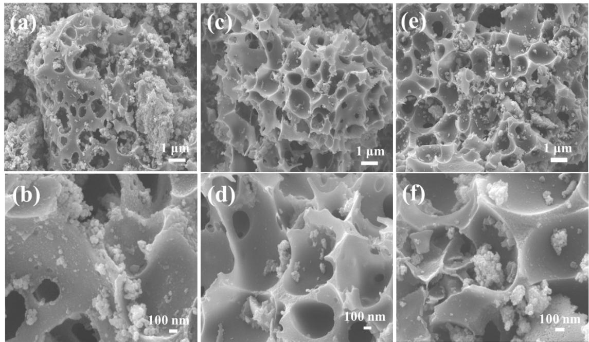
**Fig. S1.** (a) low and (b) high magnification SEM images of  $\text{Ni}_{3.5}\text{Co}_{0.5}\text{WO}_4/\text{HPC}$ ; (c) low and (d) high magnification SEM images of  $\text{Ni}_{2.5}\text{Co}_{1.5}\text{WO}_4/\text{HPC}$  and (e) low and (f) high magnification SEM images of  $\text{Ni}_2\text{Co}_2\text{WO}_4/\text{HPC}$ .
