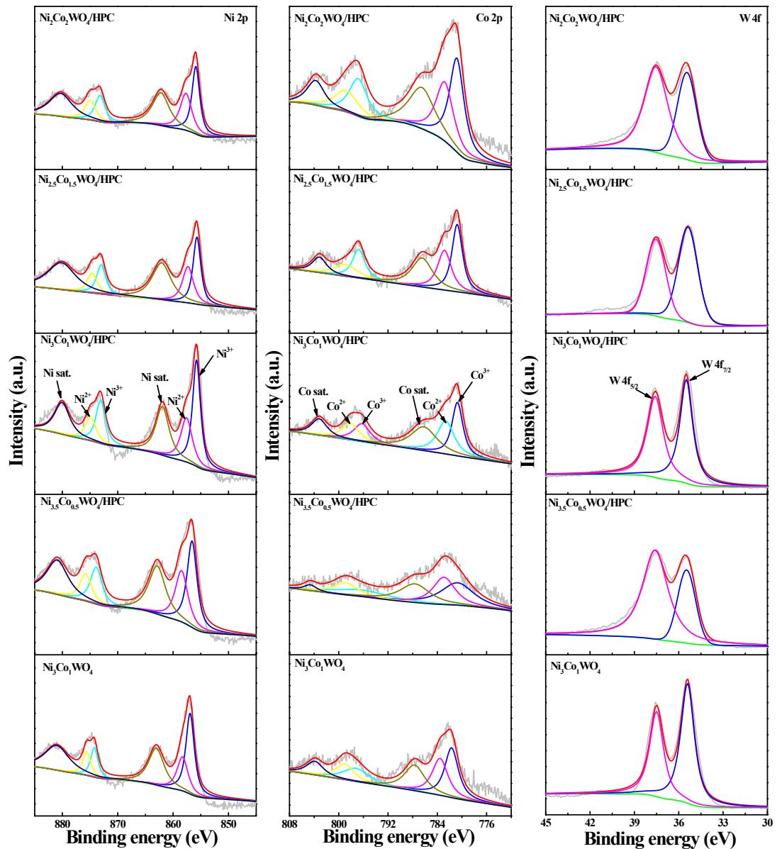
Fig. S4. High resolution XPS spectrum of Ni, Co and W in  $\text{Ni}_{4-x}\text{Co}_x\text{WO}_4/\text{HPC}$  and  $\text{Ni}_3\text{Co}_1\text{WO}_4$ .
