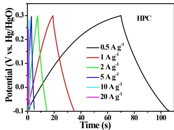
**Fig.S6.** GCD curves of HPC in a three-electrode system in 6 M KOH.
