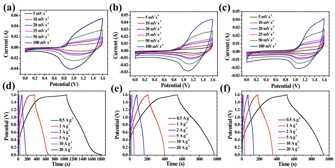
**Fig.S10.** CV curves of (a)  $\text{Ni}_{3.5}\text{Co}_{0.5}\text{WO}_4/\text{HPC}$ , (b)  $\text{Ni}_{2.5}\text{Co}_{1.5}\text{WO}_4/\text{HPC}$  and (c)  $\text{Ni}_2\text{Co}_2\text{WO}_4/\text{HPC}$ , GCD curve of (d)  $\text{Ni}_{3.5}\text{Co}_{0.5}\text{WO}_4/\text{HPC}$ , (e)  $\text{Ni}_{2.5}\text{Co}_{1.5}\text{WO}_4/\text{HPC}$  and (f)  $\text{Ni}_2\text{Co}_2\text{WO}_4/\text{HPC}$  determined in a two-electrode system in 6M KOH.
