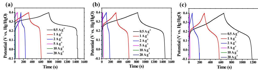
**Fig.S8.** GCD curves of (a)  $\text{Ni}_{3.5}\text{Co}_{0.5}\text{WO}_4/\text{HPC}$ , (b)  $\text{Ni}_{2.5}\text{Co}_{1.5}\text{WO}_4/\text{HPC}$  and (c)  $\text{Ni}_2\text{Co}_2\text{WO}_4/\text{HPC}$  determined in a three-electrode system in 6M KOH.
