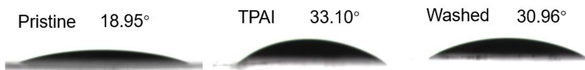
**Figure S2.** Deionized water contact angle measurements of (left) NiO<sub>x</sub>, (middle) TPAI treated NiO<sub>x</sub> film. (right) TPAI treated NiO<sub>x</sub> film washed by the DMF/DMSO mixed solvent with volume ratio of 400:37.
