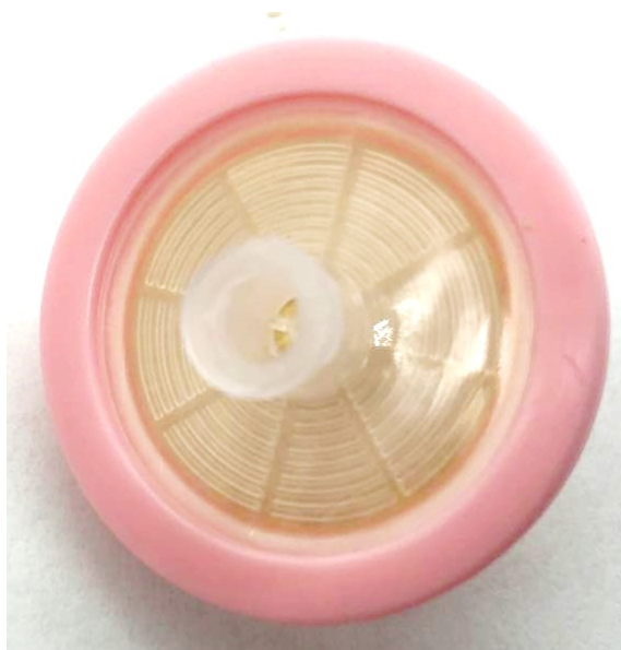
Figure S16. Mercury filter prototype produced by commercial syringe filter (a Nylon 0.45 \mu m syringe filter) with synthesized sulfur nanoparticles, SPD-50,25,05-250.
