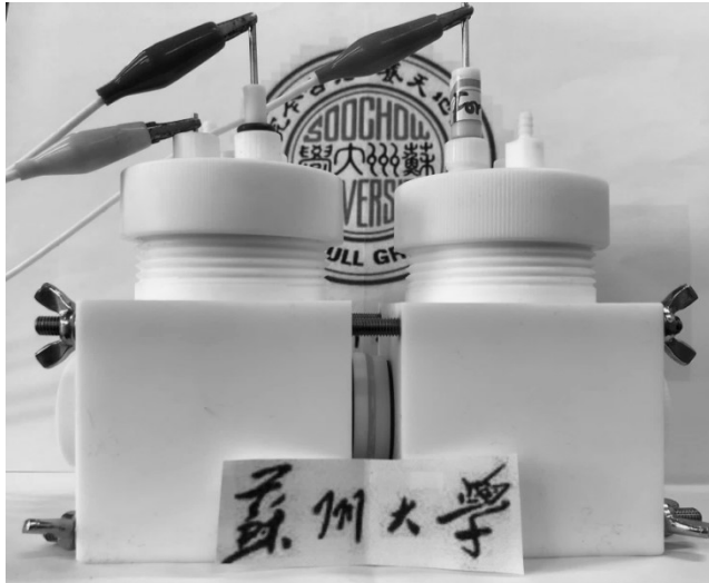
Figure S8. Photo of the PTFE made H-cell for HER and e\text{-NRA} measurements.
