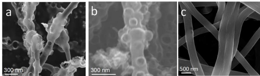
**Figure. S2.** SEM images of (a) Bi@Void⊂CNF, (b) Void@TiO<sub>2</sub>⊂CNF, and (c) pure carbon.
