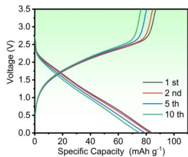
**Figure. S21.** Galvanostatic charge-discharge profiles at  $0.2 \text{ A g}^{-1}$  of Bi@Void@TiO<sub>2</sub>cnf based K-ion full cell.
