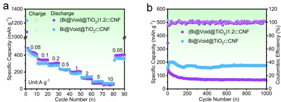
**Figure. S10.** a) Rate performance and (b) cycling performance of  $\text{Bi}@\text{Void}@\text{TiO}_2\subset\text{CNF}$  and  $(\text{Bi}@\text{Void}@\text{TiO}_2)1.2\subset\text{CNF}$  at  $2 \text{ A g}^{-1}$ .
