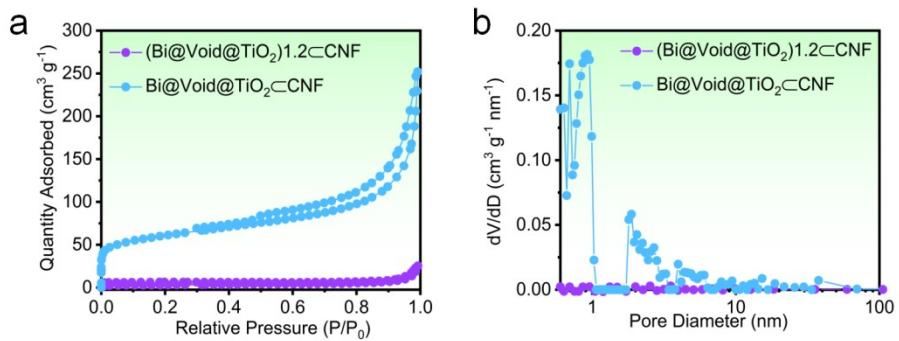
**Figure. S9.** a) Nitrogen adsorption-desorption isotherms, and (b) pore size distributions of  $(\text{Bi}@\text{Void}@\text{TiO}_2)1.2\subset\text{CNF}$ , and  $\text{Bi}@\text{Void}@\text{TiO}_2\subset\text{CNF}$ .
