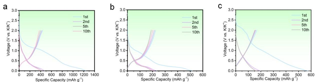
**Figure. S5.** Galvanostatic charge-discharge profiles at 0.05 A g<sup>-1</sup> of (a) Bi@Void@TiO<sub>2</sub>‐CNF, (b) Bi@Void‐CNF, and (c) Void@TiO<sub>2</sub>‐CNF.
