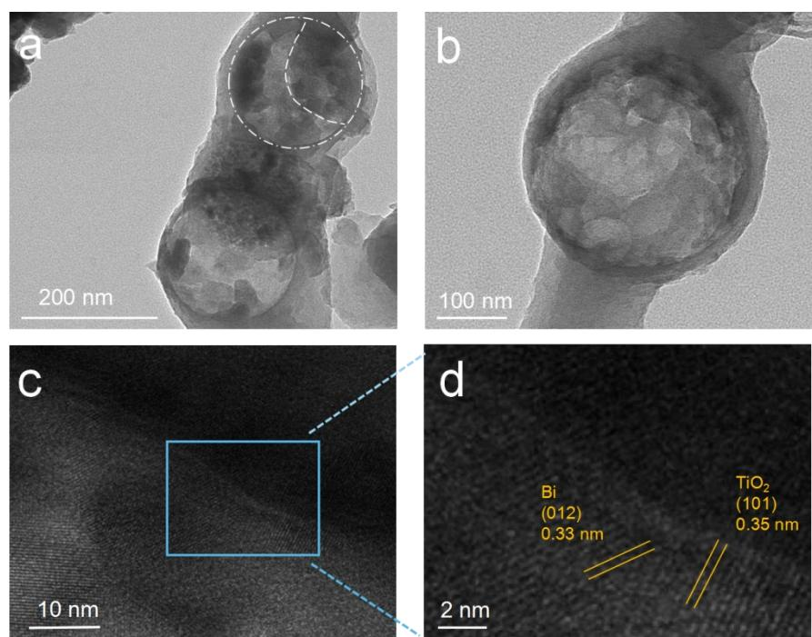
**Figure. S7.** TEM and high-resolution TEM images of Bi@Void@TiO<sub>2</sub>⊂CNF after 1000 cycles at 2 A g<sup>-1</sup>.
