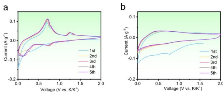
**Figure. S3.** CV curves of (a) Bi@Void⊂CNF, and (b) Void@TiO<sub>2</sub>⊂CNF at the scan rate of 0.1 mV s<sup>-1</sup>.
