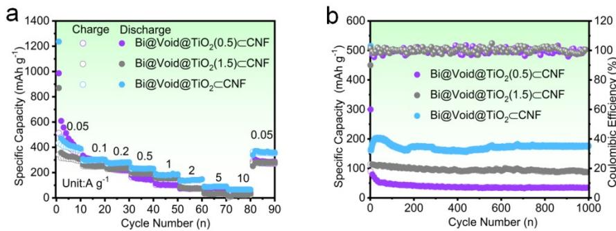
**Figure. S12.** Electrochemical performance of  $\text{Bi}@\text{Void}@\text{TiO}_2\subset\text{CNF}$ ,  $\text{Bi}@\text{Void}@\text{TiO}_2(0.5)\subset\text{CNF}$  and  $\text{Bi}@\text{Void}@\text{TiO}_2(1.5)\subset\text{CNF}$ . a) Rate performance and (b) cycling performance at  $2 \text{ A g}^{-1}$ .
