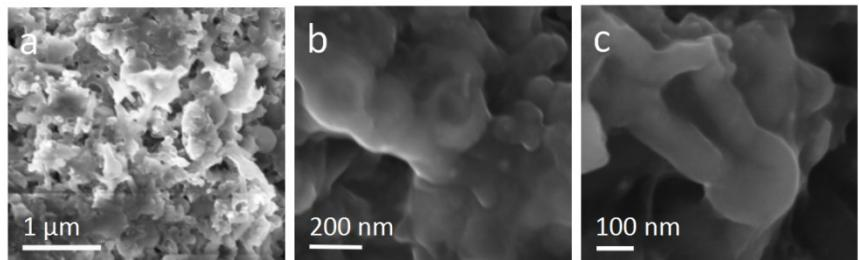
**Figure. S6.** SEM images of Bi@Void@TiO<sub>2</sub>⊂CNF after 1000 cycles at 2 A g<sup>-1</sup>.
