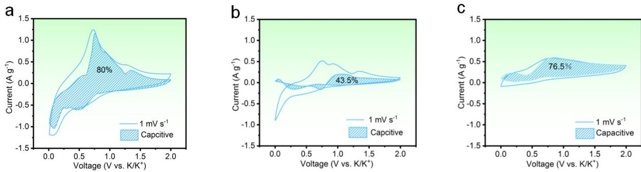
**Figure. S17.** Capacitive storage contribution (shade area) of (a) Bi@Void@TiO<sub>2</sub>⊂CNF, (b) Bi@Void⊂CNF, and (c) Void@TiO<sub>2</sub>⊂CNF at a scan rate of 1 mV s<sup>-1</sup>.
