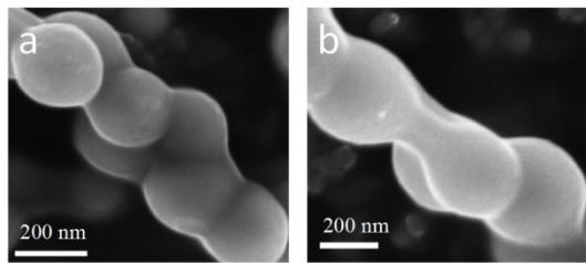
**Figure. S11.** SEM images of (a)  $\text{Bi}@\text{Void}@\text{TiO}_2(0.5)\subset\text{CNF}$  and (b)  $\text{Bi}@\text{Void}@\text{TiO}_2(1.5)\subset\text{CNF}$ .
