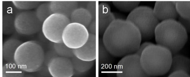
**Figure. S1.** SEM images of (a) Bi, and (b) Bi@SiO<sub>2</sub>.
