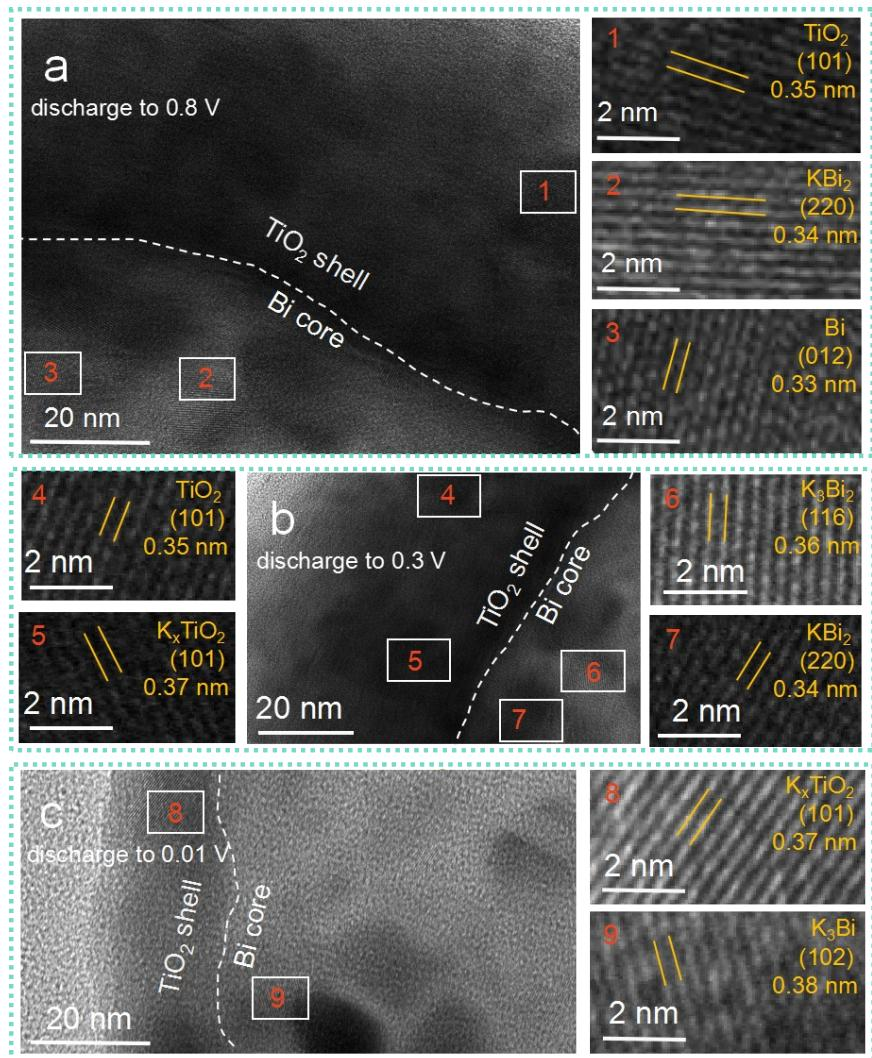
**Figure. S4.** Ex-situ high-resolution TEM images for Bi@Void@TiO<sub>2</sub>‐CNF anodes: a) after discharge to 0.8 V, b) after discharge to 0.3 V, and (c) after discharge to 0.01 V.
