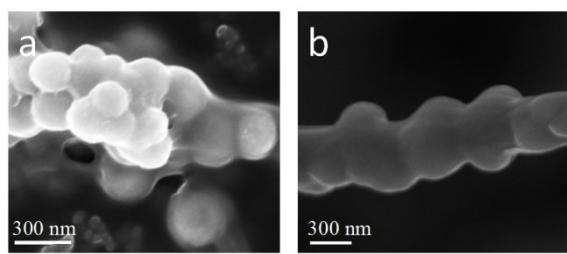
**Figure. S13.** SEM images of (a)  $\text{Bi}@\text{Void}(8)@\text{TiO}_2\subset\text{CNF}$  and (b)  $\text{Bi}@\text{Void}(12)@\text{TiO}_2\subset\text{CNF}$ .
