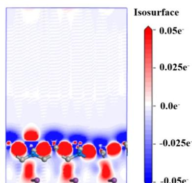
**Figure. S19.** Side view of an interlayer differential charge density diagram for a Bi/TiO<sub>2</sub> heterostructure.
