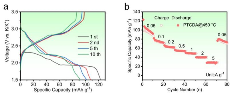
**Figure. S20.** a) Galvanostatic charge-discharge profiles at  $0.05 \text{ A g}^{-1}$ , and (b) rate cycling behavior of PTCDA@450 °C.
