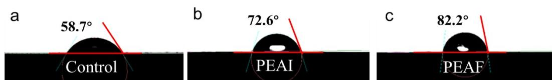
**Figure S18.** Images of water droplets between water and pristine (a), PEAI-treated (b) and PEAf-treated perovskite films.
