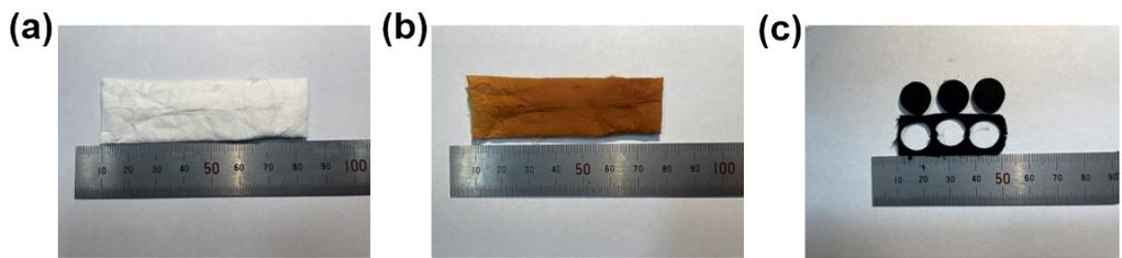
**Figure S3.** Digital images of (a) PAN membrane, (b) pre-oxidized membrane, (c) carbonized membrane and self-supported cathodes.
