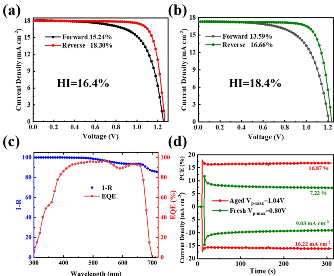
**Figure S9** J-V curves of the (a) aged and (b) fresh PSCs measured with different scan directions. HI is defined according to the equation:  $HI = (PCE_{Reverse} - PCE_{Forward}) / PCE_{Reverse} \times 100\%$ ; (c) EQE and 1-R curves of the aged PSC. (d) Steady-state output of the fresh and aged PSCs under the voltages at maximum power points of 0.80 V and 1.04 V, respectively.
