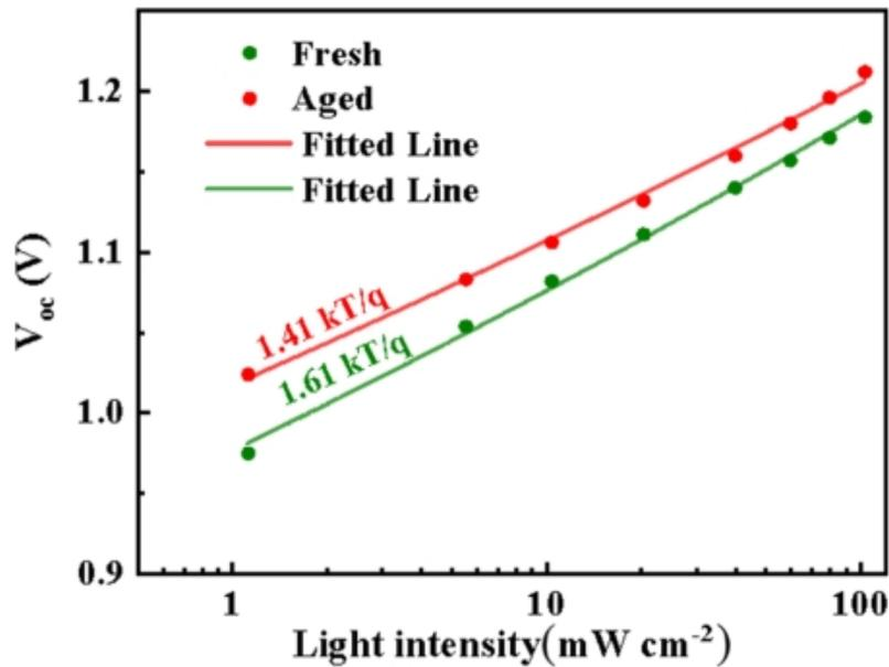
**Figure S12** Light-dependent  $V_{oc}$  measurement.
