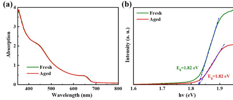
**Figure S1** (a) UV-vis absorption spectra and (b) Energy bandgap of the fresh and aged perovskite films.
