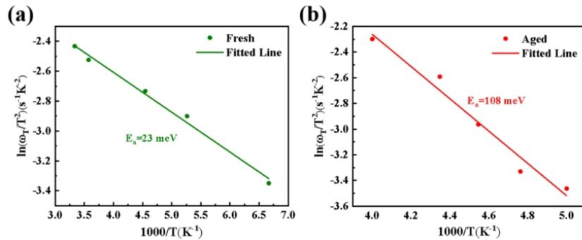
**Figure S3** Arrhenius plot extracted from the derivative peak of  $\omega(dC/d\omega)$  versus  $\omega$  plot at low-frequency region for (a) Fresh; (b) Aged devices.
