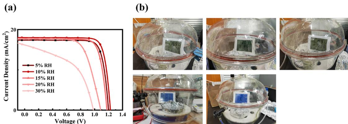
**Figure S8.** (a) J–V characteristics of the PSCs fabricated from the aging process with different humidity conditions; (b) Photographs of the storage boxes used for controlling the humidity.
