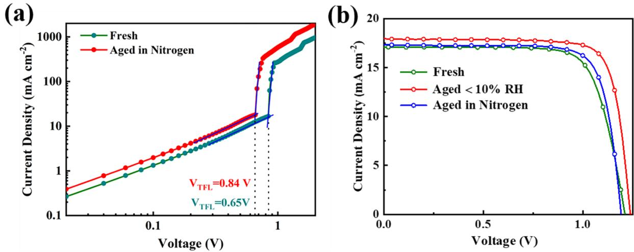
**Figure S6.** (a) J–V curves of electron-only devices for the fresh and aged film in an inert  $N_2$  gas condition; (b) Typical J–V curves of  $CsPbI_{3-x}Br_x$  PSCs aged in a low humidity condition and in an inert  $N_2$  gas condition.
