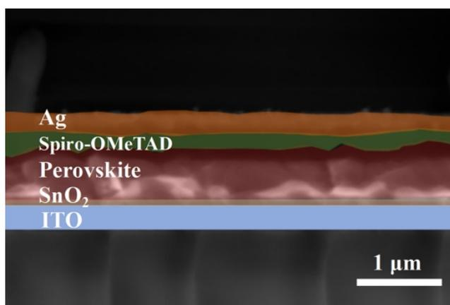
**Figure S5** Cross-section SEM image of the CsPbI<sub>3-x</sub>Br<sub>x</sub> PSC.
