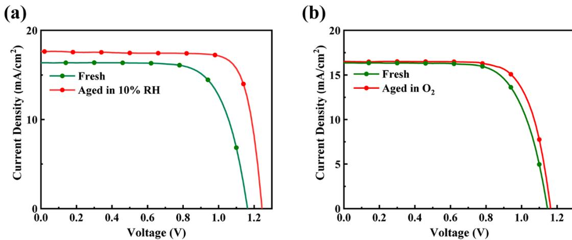
**Figure S7.** Comparison of the  $CsPbI_{3-x}Br_x$  PSCs fabricated with the aging process conducted in different conditions. (a) Aged in 10% RH condition, (b) Aged in  $O_2$  condition.
