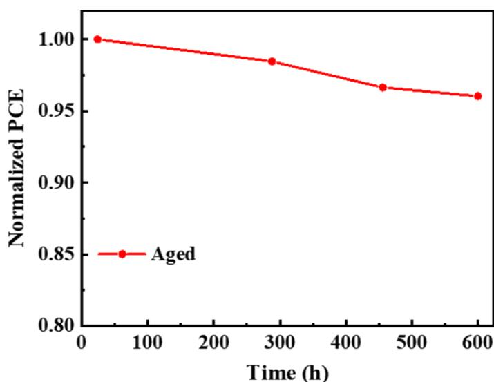
**Figure S10** PCE evolution of the unencapsulated device under ~30% RH at room temperature in ambient condition.
