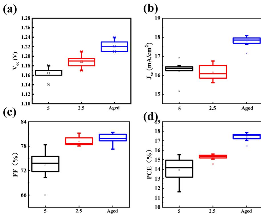
**Figure S4.** The statistical data of the CsPbI<sub>3-x</sub>Br<sub>x</sub> PSCs with 5  $\mu$ l, 2.5  $\mu$ l water as an additive in the inorganic perovskite precursor. The data of the aged devices is given for comparison. (a)  $V_{oc}$ ; (b)  $J_{sc}$ ; (c) FF; (d) PCE
