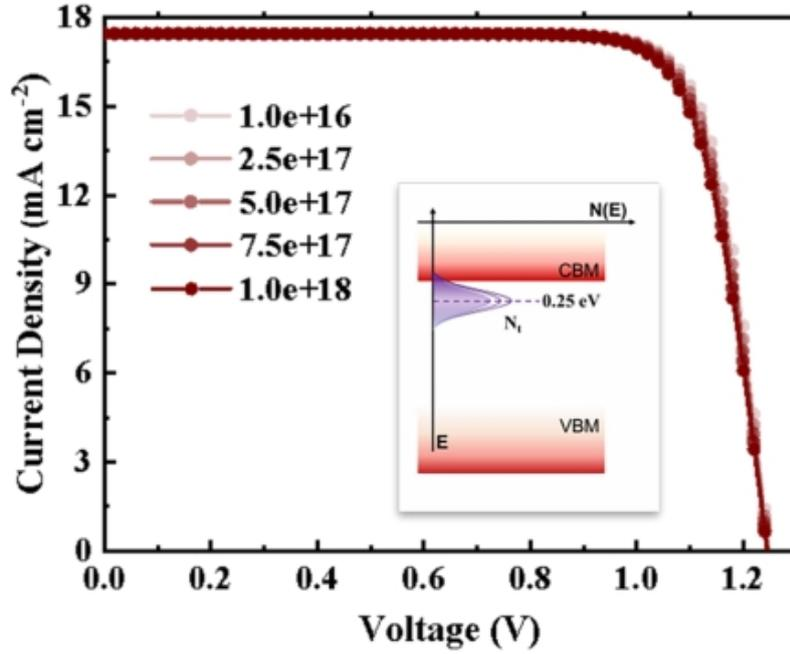
**Figure S11** Device simulation using SCAPS for the CsPbI<sub>3-x</sub>Br<sub>x</sub> PSC with different shallow-level defect densities. The  $E_a$  of the shallow-level defect is 0.25 eV.
