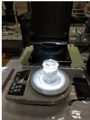
Fig. S16 Photograph of the solar evaporator setup.
