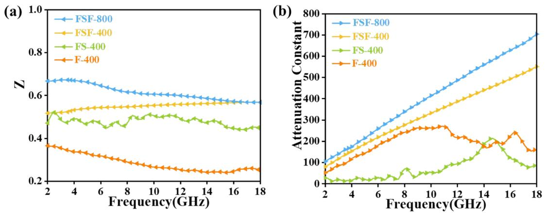
Fig. S5 (a) Impedance matching constant ( $Z$ ) and (b) attenuation constant ( $\alpha$ ) of the composites.
