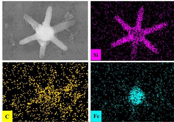
**Fig. S1** EDS elemental mapping of FSF-0
