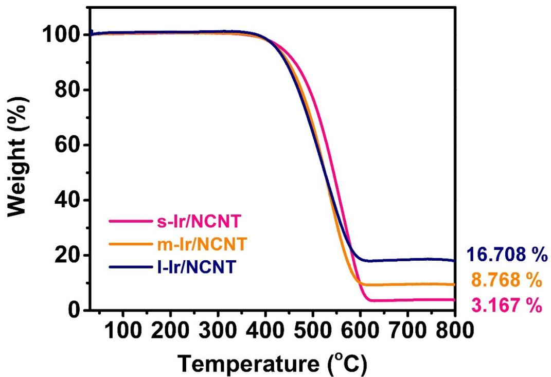
**Figure S3.** TGA curves of s-, m- and l-Ir/NCNTs in the temperature range of 30–800 °C at a heating rate of 10 °C/min in air.
