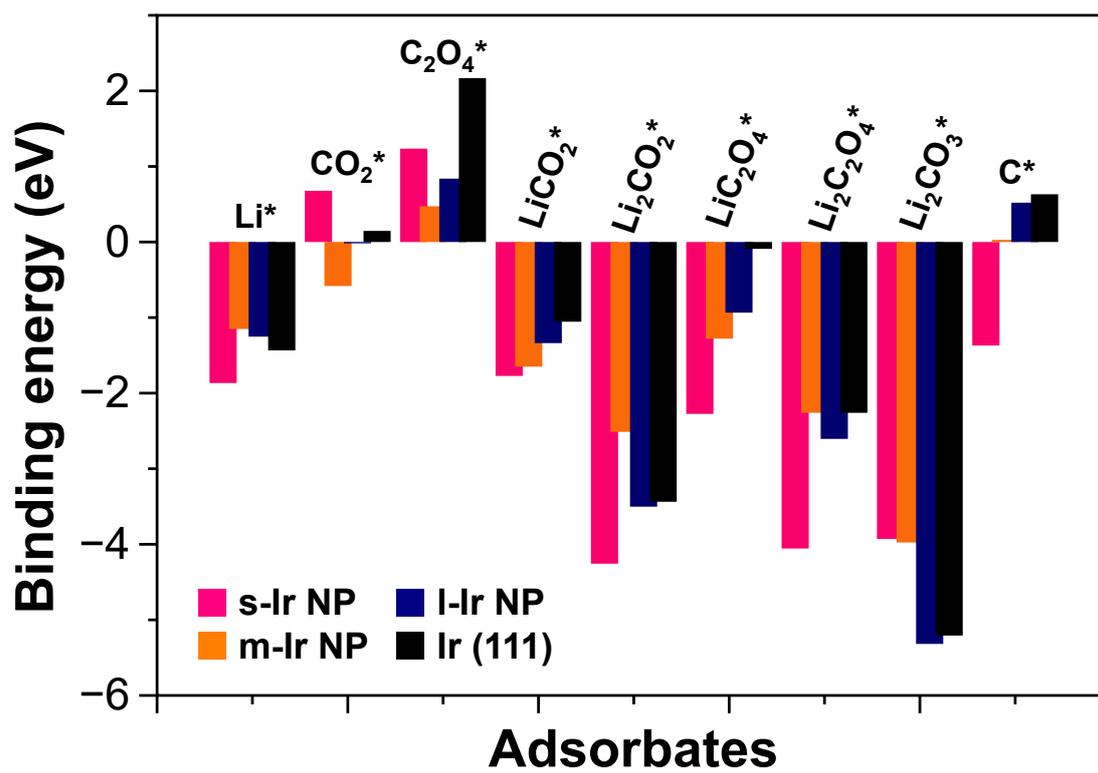
Figure S10. Binding energies of intermediates on the different Ir particle systems.
