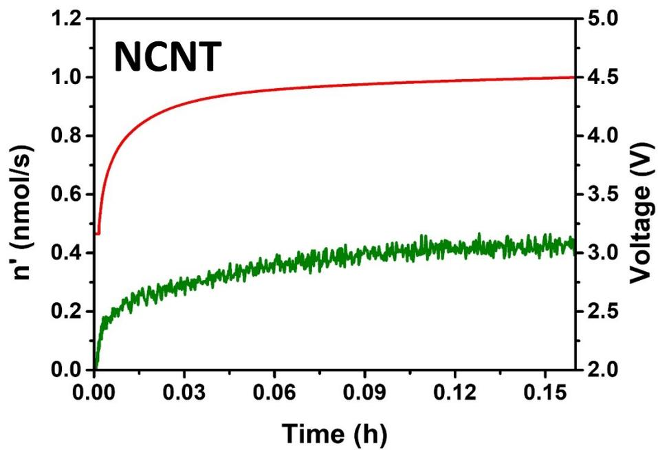
**Figure S7.** *In situ* DEMS results of the rate of evolution of CO<sub>2</sub> during charging in cells employing NCNTs.
