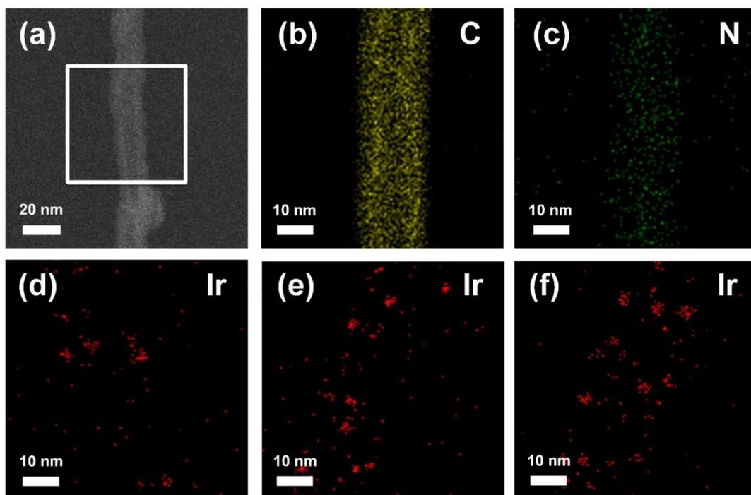
**Figure S4.** (a) STEM image and EDS mappings of (b) C and (c) N in NCNT and Ir in (d) s-Ir/NCNT, (e) m-Ir/NCNT and (f) l-Ir/NCNT.
