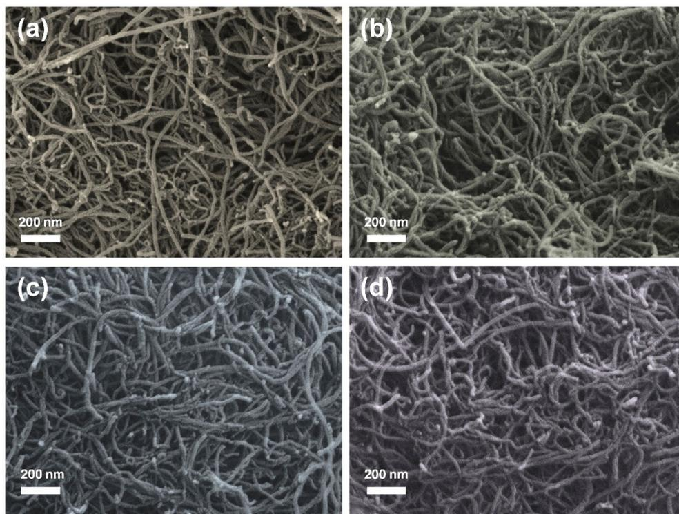
**Figure S1.** SEM images of (a) NCNT, (b) s-Ir/NCNT, (c) m-Ir/NCNT, and (d) l-Ir/NCNT.
