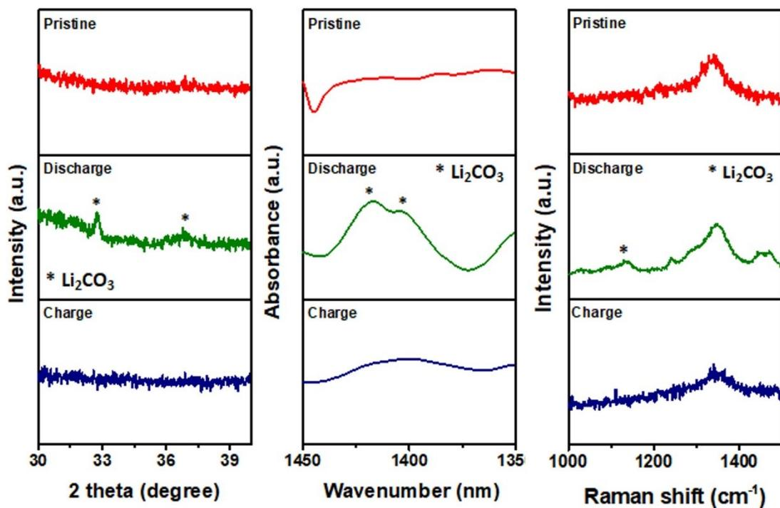
**Figure S8.** *Ex situ* measurements on carbon electrodes. XRD, FT-IR and Raman peaks obtained from discharged and charged electrodes of s-Ir/NCNT.
