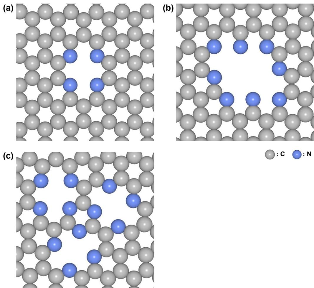
**Figure S5.** Illustration of base structures for (a) IrO<sub>x</sub>/Ir SAC (or IrO<sub>2</sub> SAC), (b) m-Ir NP (or Ir<sub>6</sub> NP), and (c) l-Ir NP (or Ir<sub>12</sub> NP).
