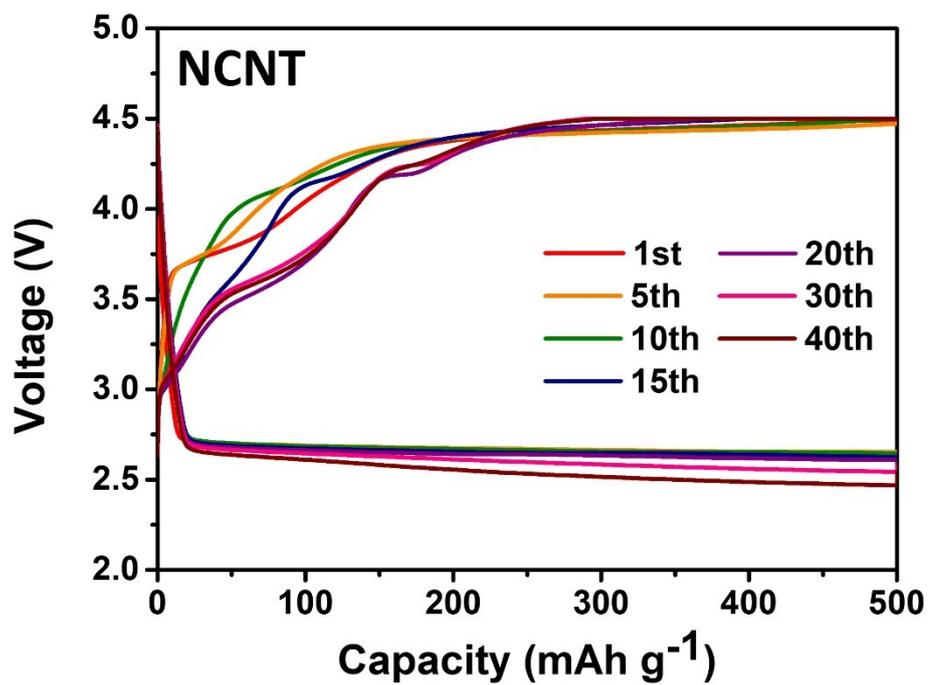
**Figure S6.** Cycling performance of Li-CO<sub>2</sub> cells employing NCNTs in the 2.3–4.5 V voltage window under the specific capacity limit of 500 mAh g<sub>carbon</sub><sup>-1</sup>.
