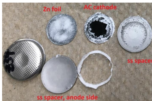
Figure S12. (a) Comparison of specific capacity of an Aq ZIC before and after reassembly. After the Aq ZIC died during the rate test (~ 45 cycles), the coin cell was opened and the AC cathode was retrieved. The same AC cathode but fresh electrolyte, separator, Zn foil, and coin cell components were used for the reassembly (new cell). The slight difference in the capacity could be because of a slight change in the density of the cathode as a result of experiencing compression during coin cell opening and reassembly. The mass loading of AC30 in the cathode is 2.35 mg/cm 2 (ZIC with 2M ZnSO 4 ). (b) The photo of the disassembled components of the Aq ZIC in (a) after cell failure, in which no yellowish color (iron rust) was observed.
