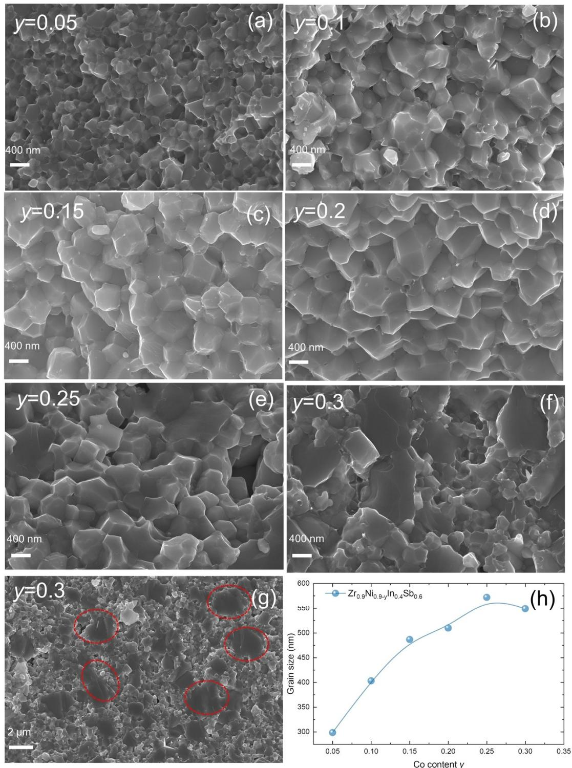
Fig. S2 The SEM images for (a)  $y=0.05$ , (b)  $y=0.1$ , (c)  $y=0.15$ , (d)  $y=0.2$ , (e)  $y=0.25$ , and (f) - (g)  $y=0.3$  in  $\text{Zr}_{0.9}\text{Ni}_{0.9-y}\text{Co}_y\text{In}_{0.4}\text{Sb}_{0.6}$  and (h) Co-content dependence of grain size.
