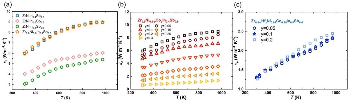
Fig. S4 Temperature dependence of  $\kappa_e$  for  $\text{ZrNiIn}_x\text{Sb}_{1-x}$ ,  $\text{Zr}_{0.9}\text{Ni}_{0.9-y}\text{Co}_y\text{In}_{0.4}\text{Sb}_{0.6}$  and  $\text{Zr}_{0.9-z}\text{Hf}_z\text{Ni}_{0.625}\text{Co}_{0.25}\text{In}_{0.4}\text{Sb}_{0.6}$  samples.
