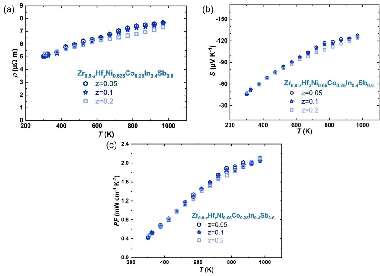
Fig. S3 Temperature dependence of electrical properties for  $\text{Zr}_{0.9-z}\text{Hf}_z\text{Ni}_{0.625}\text{Co}_{0.25}\text{In}_{0.4}\text{Sb}_{0.6}$  ( $z = 0.05 - 0.2$ )
