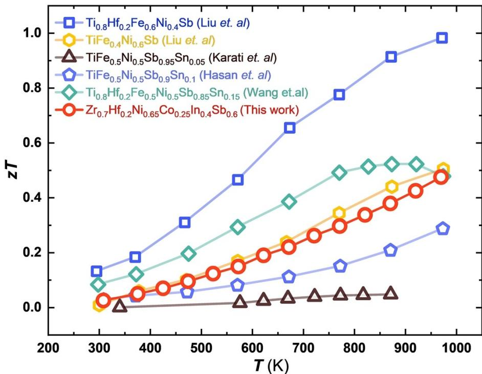
Fig. S5 Comparison of temperature dependence of  $zT$  for reported double HH compounds<sup>1-4</sup>.
