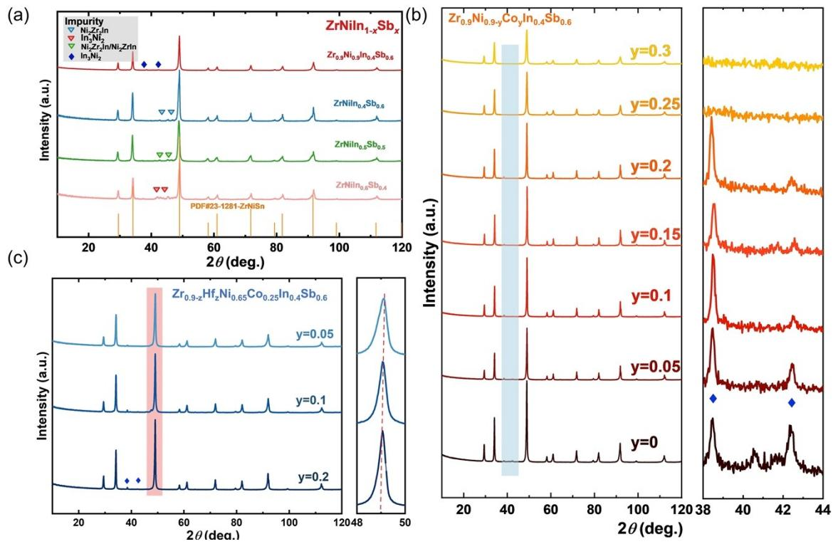
Fig. S1 XRD patterns of  $\text{ZrNiIn}_x\text{Sb}_{1-x}$ -based materials.
