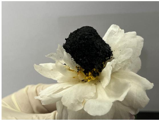
**Fig. S1.** 1T-WS<sub>2</sub>/CNT/rGO Aerogel.
