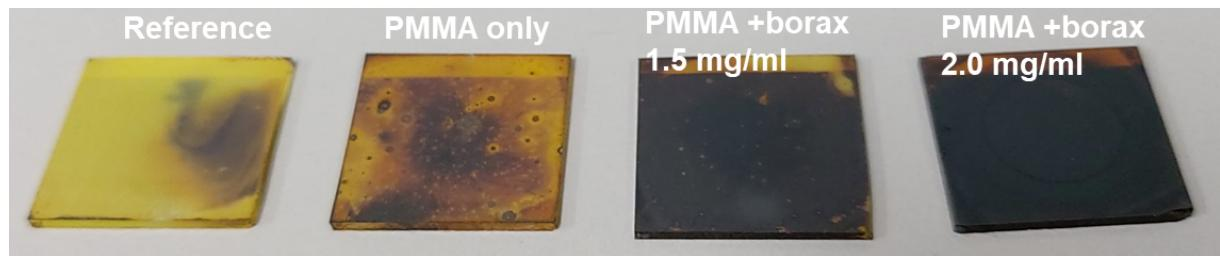
**Figure S12.** Images of the degraded as-prepared perovskite samples at 25 °C, 20 ± 10% humidity, obtained after 30 d (reference, PMMA-only, PMMA + borax (1.5 mg/mL), PMMA + borax (2.0 mg/mL) samples).
