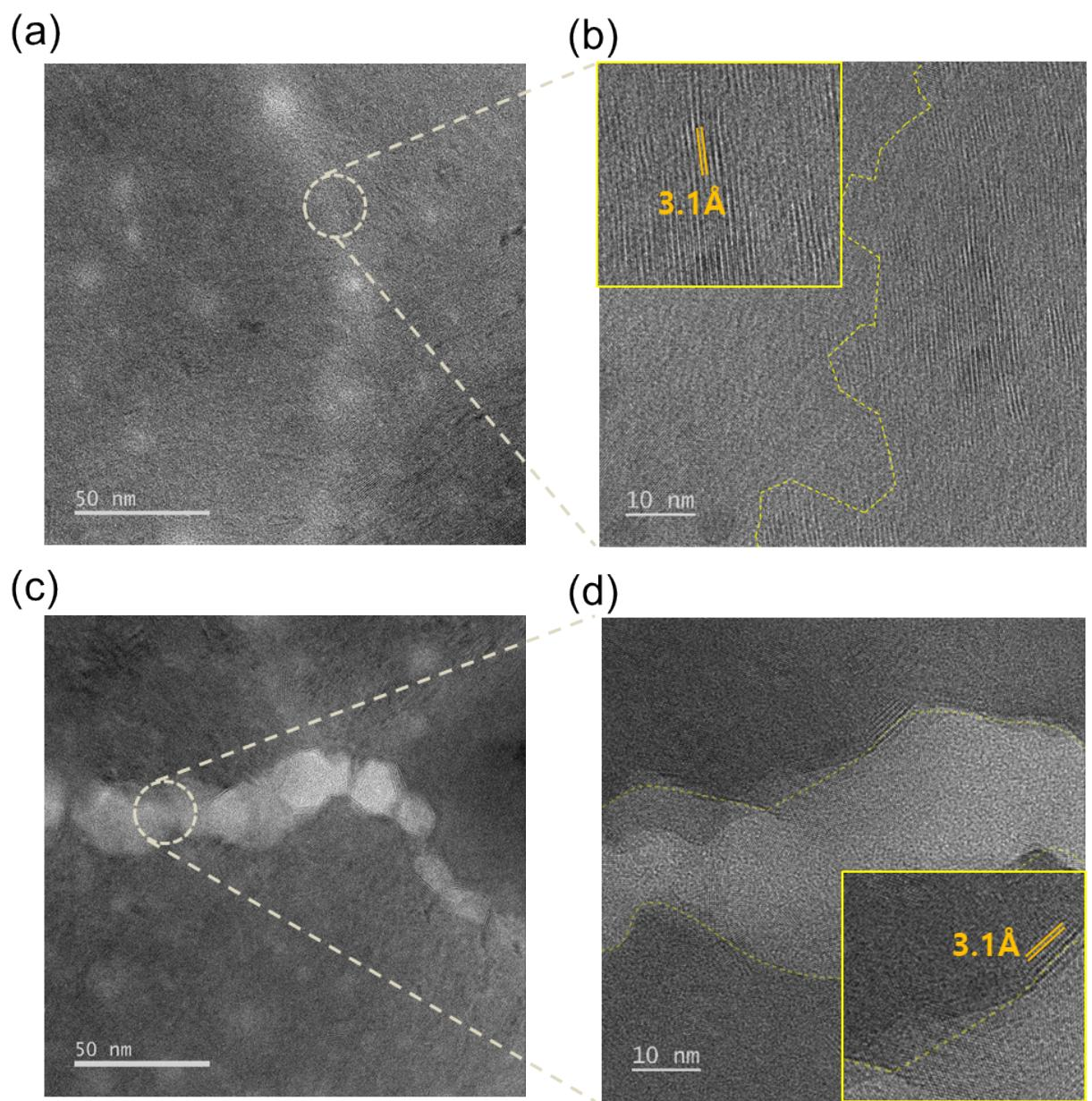
**Figure S2.** TEM images of the GBs of the (a, b) reference sample and (c, d) PMMA + borax (2.0 mg/mL) sample.
