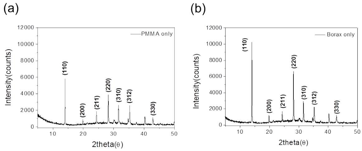
**Figure S9.** XRD spectra of the (a) PMMA-only and (b) borax-only perovskite films.
