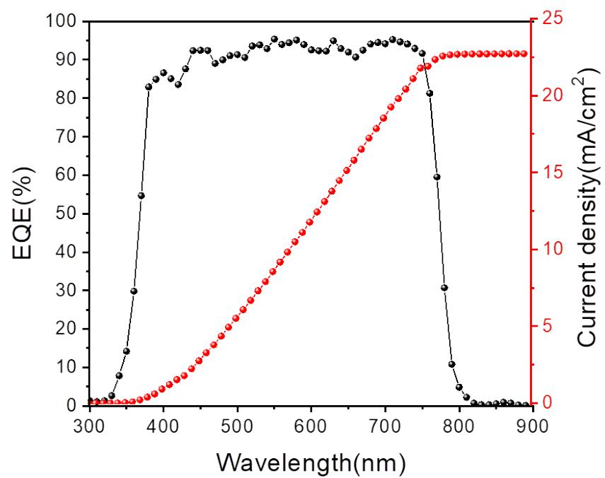
**Figure S6.** Measured EQE of the PSCs with PMMA/borax mixture ([PMMA] = 0.3 mg/mL, [borax] = 3 mg/mL).
