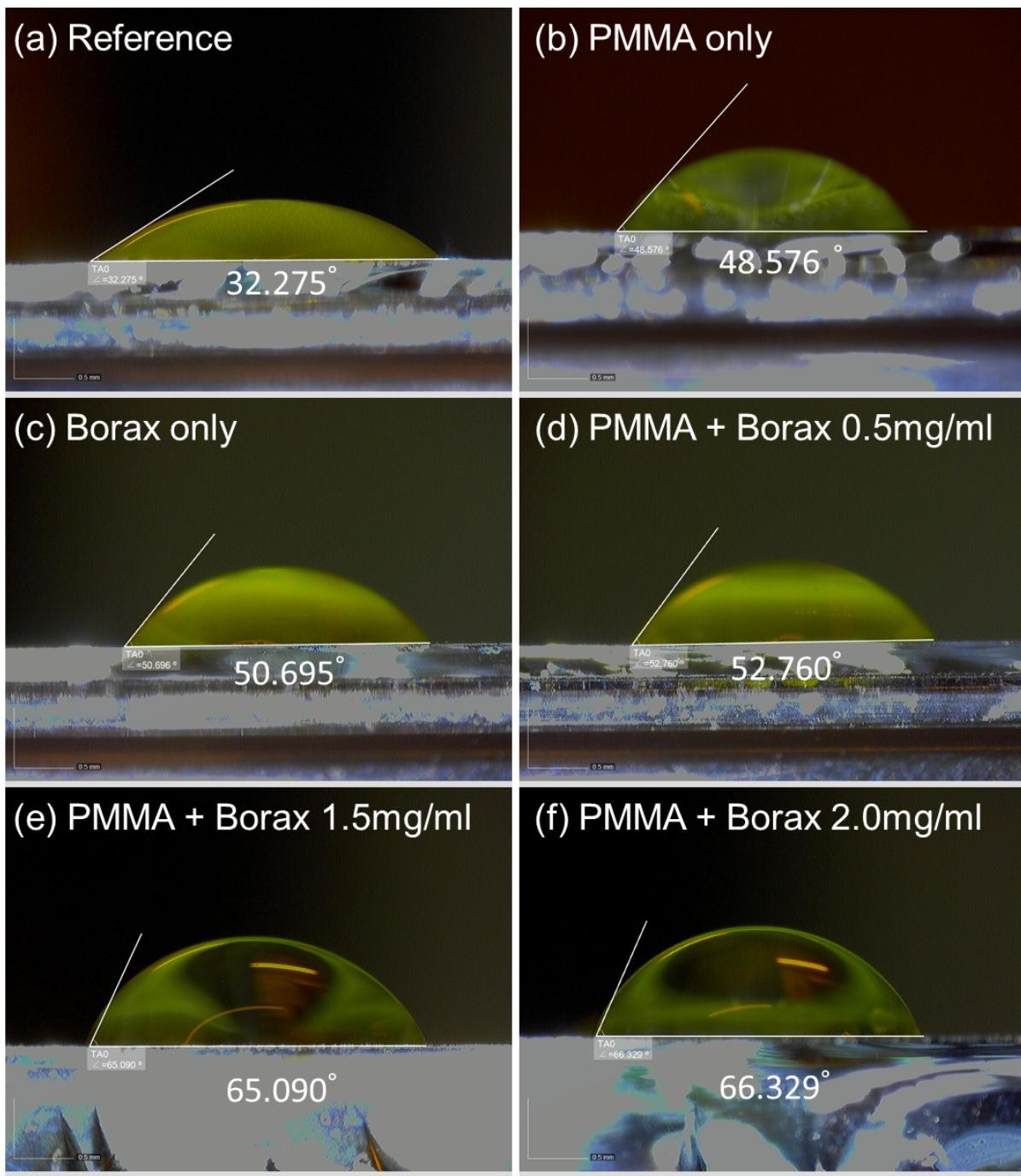
**Figure S11.** Contact angles of deionized water droplets on the (a) reference sample, (b) PMMA-only sample, (c) borax-only sample, (d) PMMA (0.3 mg/mL)/borax (0.5 mg/mL) sample, (e) PMMA (0.3 mg/mL)/borax (1.5 mg/mL) sample, and (f) PMMA (0.3 mg/mL)/borax (2.0 mg/mL) sample.
