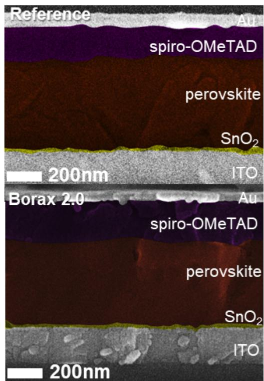
**Figure S3.** Cross sectional FE-SEM image of the full structure of reference and PMMA/borax mixture ([PMMA] = 0.3 mg/mL, [borax] = 3 mg/mL) PSCs.
