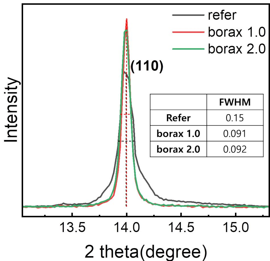
Figure S1. Comparison of FWHM values of reference, borax 1.0, and borax 2.0 samples.
