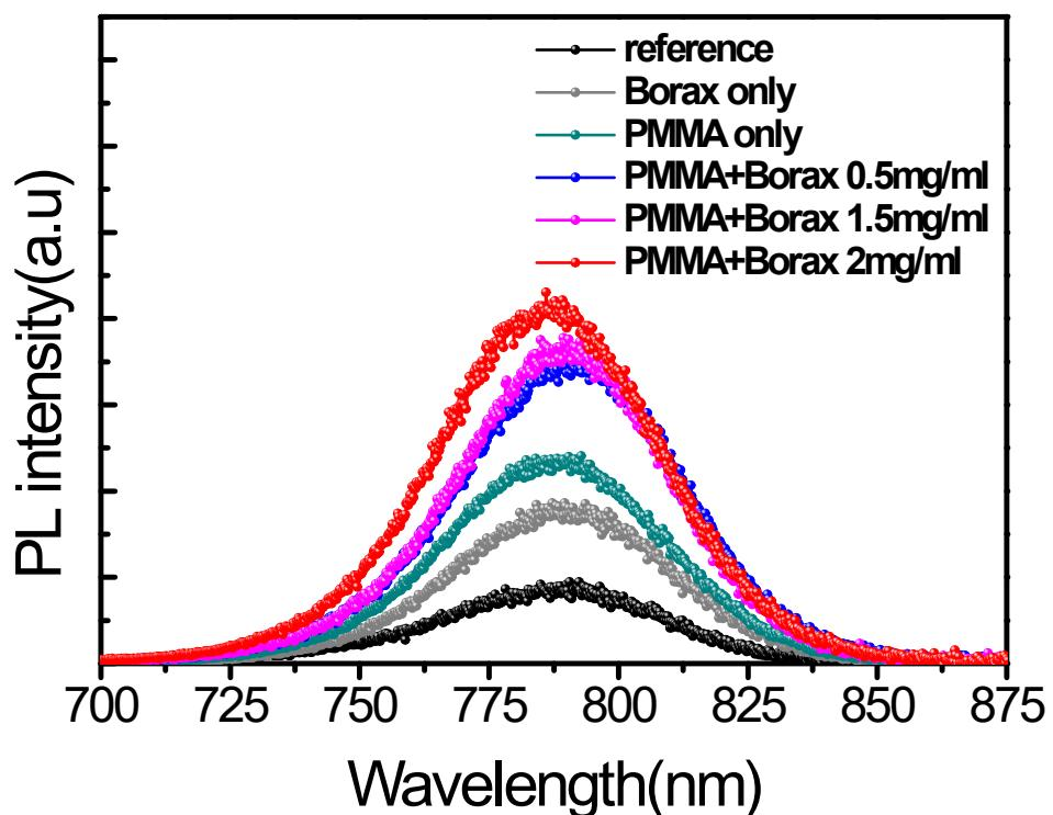
**Figure S8.** Steady-state PL spectra of the PSCs with various concentrations of additives (reference, borax-only, PMMA-only, PMMA (0.3 mg/mL)/borax (0.5, 1.5, 2.0 mg/mL) samples).
