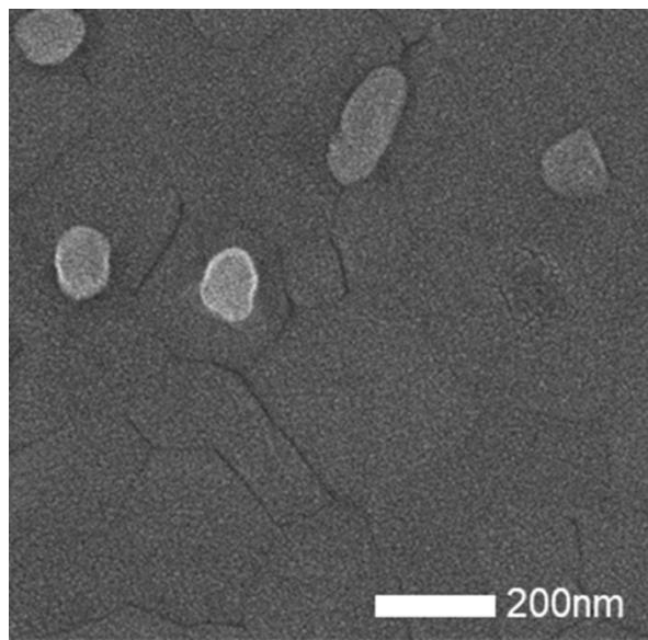
**Figure S5.** Top FE-SEM image of the PMMA/borax mixture ( $[PMMA] = 0.3\text{ mg/mL}$ ,  $[borax] = 3\text{ mg/mL}$ ).
