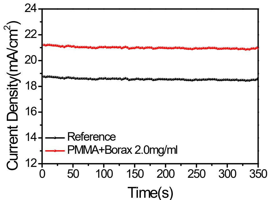
**Figure S7.** PCEs measured at the maximum power point of the PSCs with and without PMMA/borax additives.
