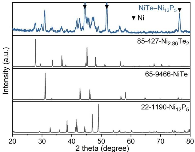
**Figure S3.** XRD pattern of NiTe–Ni<sub>12</sub>P<sub>5</sub> on NF and simulated patterns of Ni<sub>12</sub>P<sub>5</sub>, NiTe and Ni<sub>2.86</sub>Te<sub>2</sub>.
