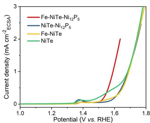
**Figure S10.** ECSA-normalized LSV curves of Fe-NiTe–Ni<sub>12</sub>P<sub>5</sub>, NiTe–Ni<sub>12</sub>P<sub>5</sub>, Fe-NiTe and NiTe.
