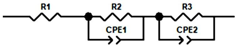
**Figure S11.** The equivalent circuit diagram used for EIS fitting.
