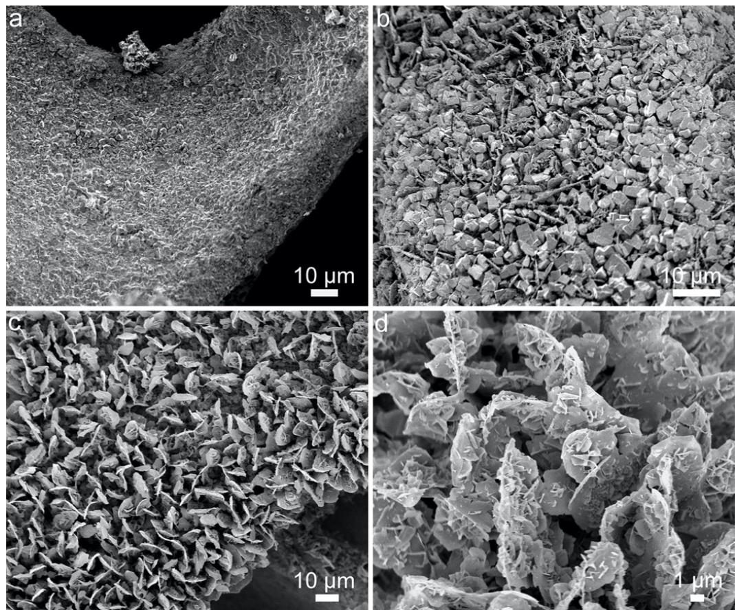
**Figure S4.** SEM images of (a, b) NiTe–Ni<sub>12</sub>P<sub>5</sub> and (c, d) NiTe grown on the NF substrate.
