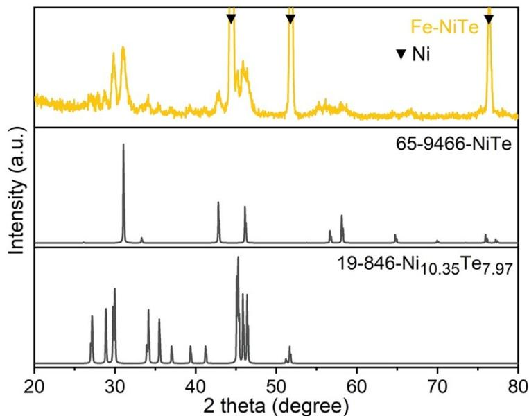
**Figure S1.** XRD pattern of Fe-NiTe on NF and simulated patterns of NiTe and Ni<sub>10.35</sub>Te<sub>7.97</sub>.
