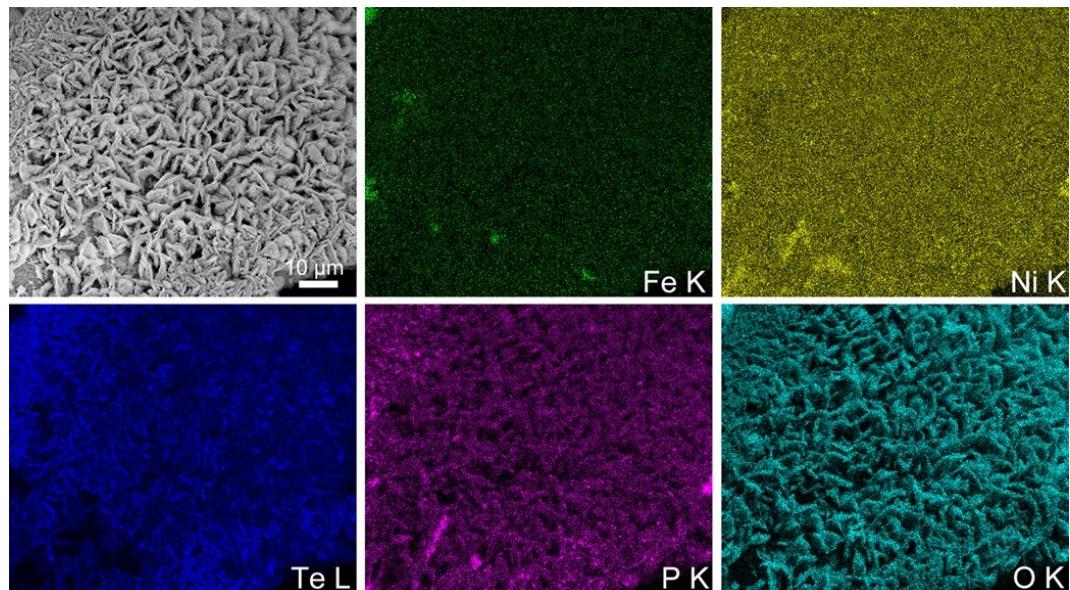
**Figure S15.** Elemental mapping images of Fe-NiTe–Ni<sub>12</sub>P<sub>5</sub> on NF after the 5000 CV cycles stability test.
