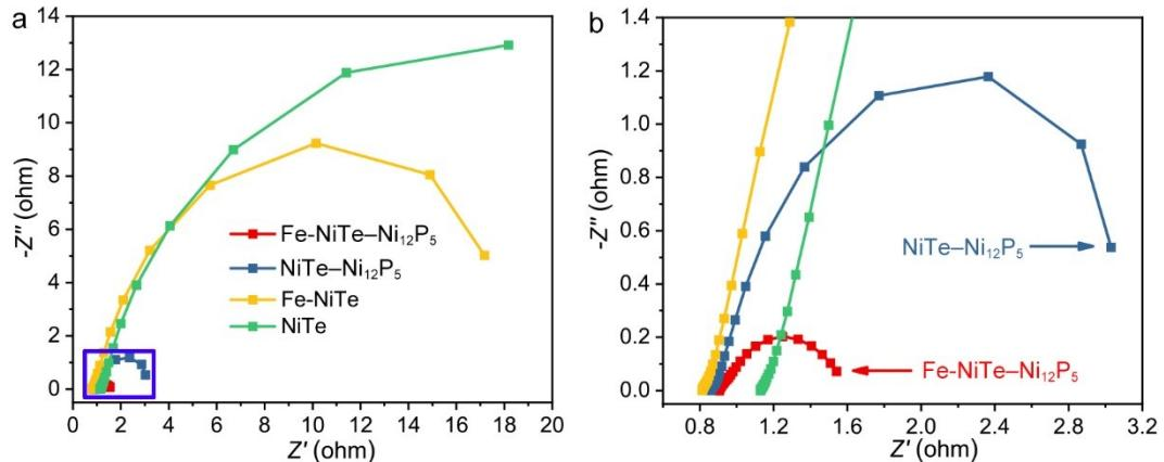
**Figure S12.** (a) EIS of four samples including Fe-NiTe-Ni<sub>12</sub>P<sub>5</sub>, NiTe-Ni<sub>12</sub>P<sub>5</sub>, Fe-NiTe and NiTe measured at the overpotential of 300 mV in an alkaline medium. (b) The magnified plot of the marked region of (a) in blue.
