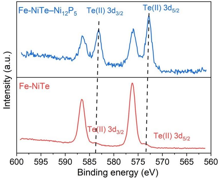
**Figure S17.** Te 3d XPS spectra of Fe-NiTe and Fe-NiTe–Ni<sub>12</sub>P<sub>5</sub>.
