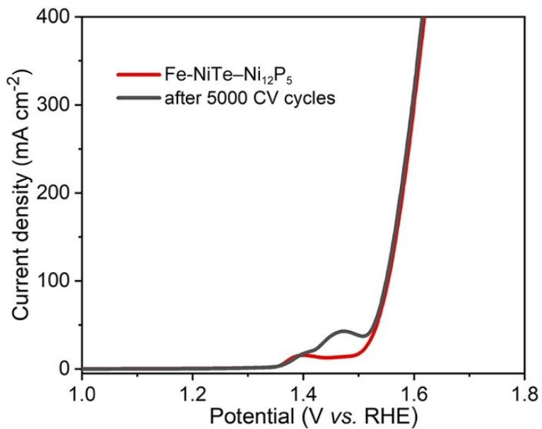
**Figure S13.** LSV curves of Fe-NiTe-Ni<sub>12</sub>P<sub>5</sub> before and after 5000 CV cycles stability test in 1.0 M KOH.
