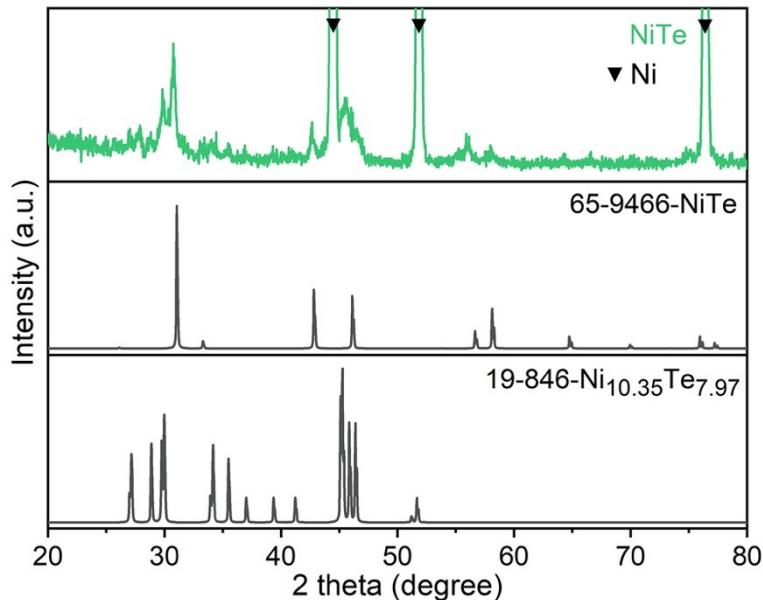
**Figure S2.** XRD pattern of NiTe on NF and simulated patterns of NiTe and Ni<sub>10.35</sub>Te<sub>7.97</sub>.
