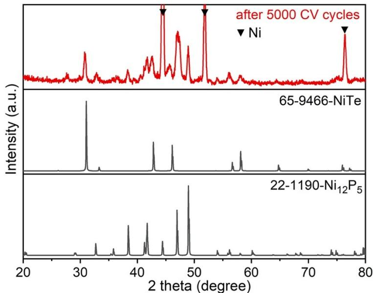
**Figure S14.** XRD pattern of Fe-NiTe–Ni<sub>12</sub>P<sub>5</sub> on NF after the 5000 CV cycles stability test and simulated patterns of NiTe and Ni<sub>12</sub>P<sub>5</sub>.
