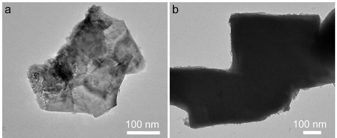
**Figure S5.** TEM images of Fe-NiTe–Ni<sub>12</sub>P<sub>5</sub> ultrasonicated from NF.
