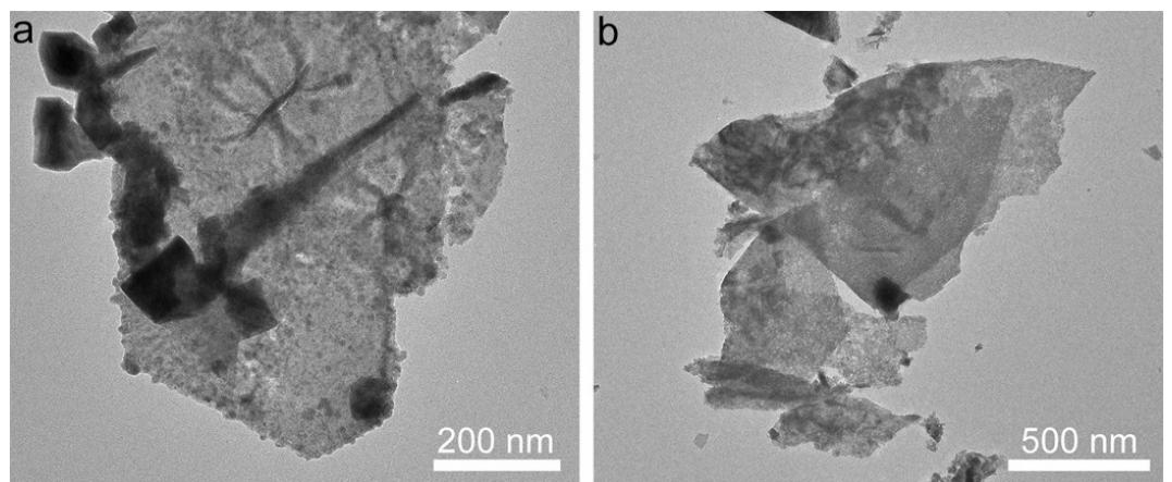
**Figure S6.** TEM images of (a, b) NiTe–Ni<sub>12</sub>P<sub>5</sub> and (c, d) NiTe ultrasonicated from the NF substrate.
