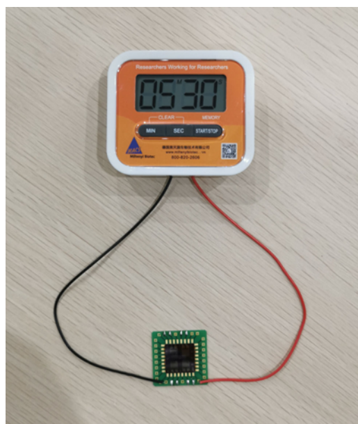
Figure S23. Photographs of 3D MSCs in series powering a timer.
