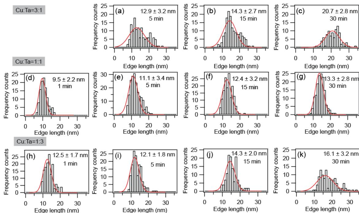
**Figure S5.** Particle size distribution histogram of (a-c) Cu:Ta=3:1 for 5 min, 15 min, and 30 min reactions and (d-g) Cu:Ta=1:3 for 1 min, 5 min, 15 min, and 30 min reactions. The average edge length and the half width half maximum is mentioned in the figure.
