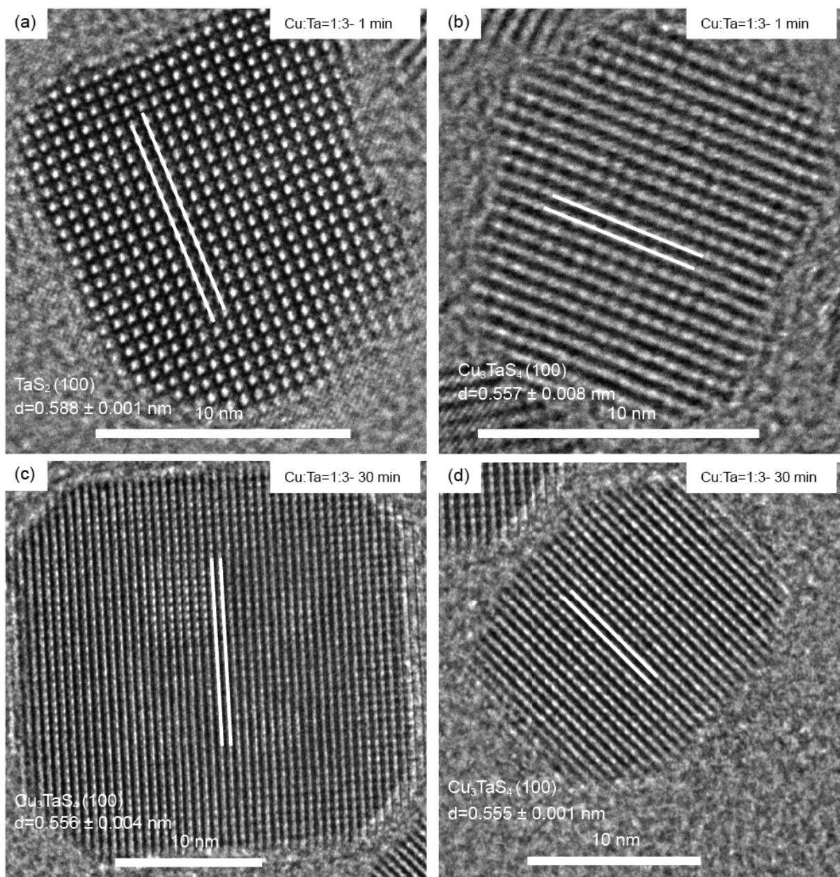
**Figure S6.** HRTEM images of the synthesized NCs for Cu:Ta=1:3 ratio. (a-b) Two individual particles after 1 min reaction. (c-d) 30 min reaction.
