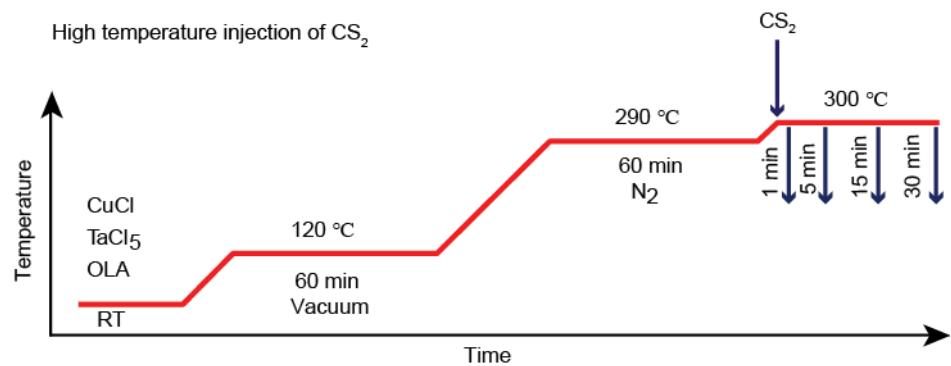
**Figure S1.** The schematic of the synthesis of copper tantalum sulfide nanocrystals for high temperature injection of CS<sub>2</sub>.
