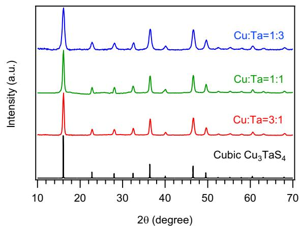
**Figure S2.** PXRD pattern of the synthesized NCs for Cu:Ta=3:1, 1:1, and 1:3 reactions. In all three cases, the NCs are crystallizes in cubic phase Cu<sub>3</sub>TaS<sub>4</sub>.
