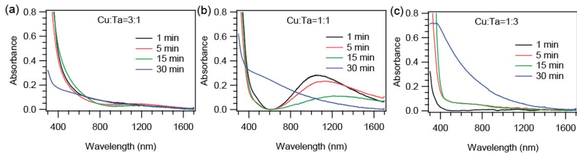
**Figure S4.** Absorption spectra of the synthesized NCs for (a) Cu:Ta=3:1, (b) Cu:Ta=1:1, (c) Cu:Ta=1:3 reactions after 1 min, 5 min, 15 min, and 30 min.
