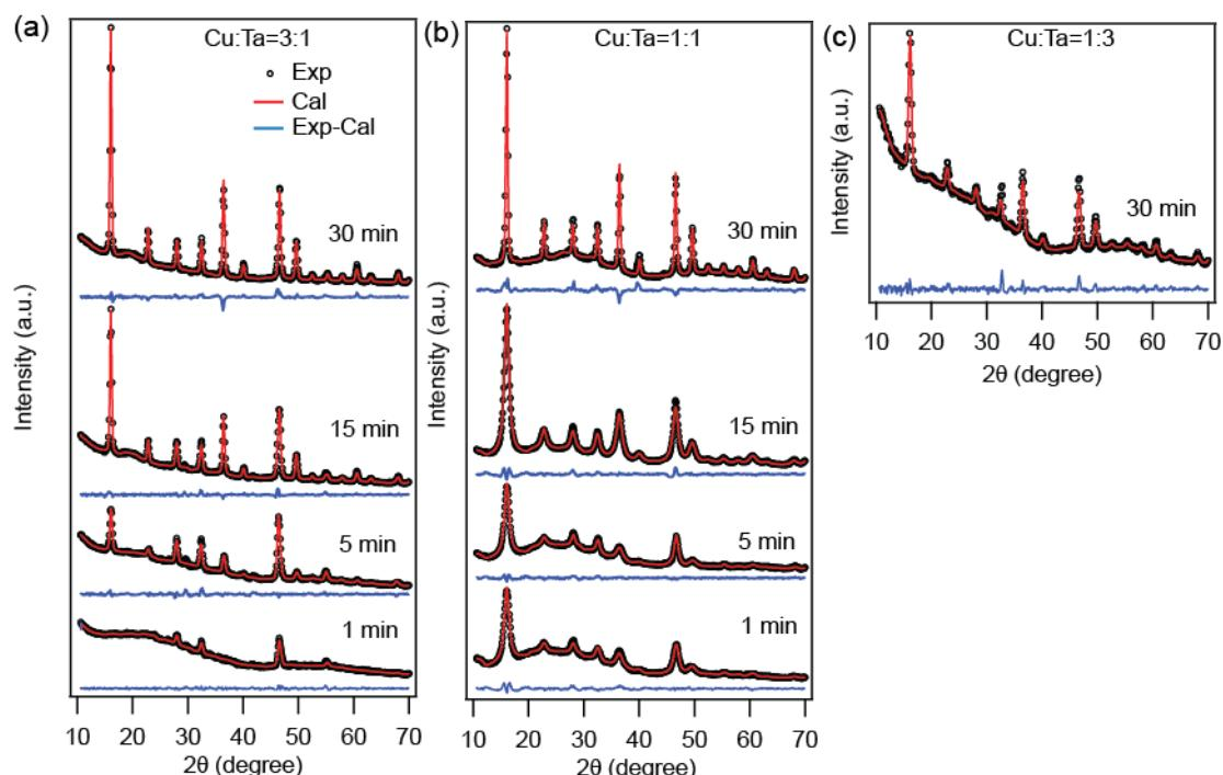
**Figure S3.** Rietveld refinement profile for (a)  $\text{Cu:Ta}=3:1$ , (b)  $\text{Cu:Ta}=1:1$ , and (c)  $\text{Cu:Ta}=1:3$  reactions. XRD patterns are vertically shifted for representing data at different reaction times. The black open circles represent the experimental XRD pattern, red solid line is calculated pattern, and the blue line is the difference between the observed and calculated XRD pattern.
