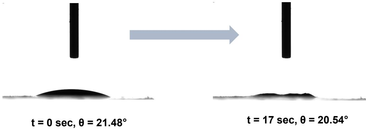
**Figure S5.** Contact angle measurement of the 5 wt% SWCNT nanocomposite material.
