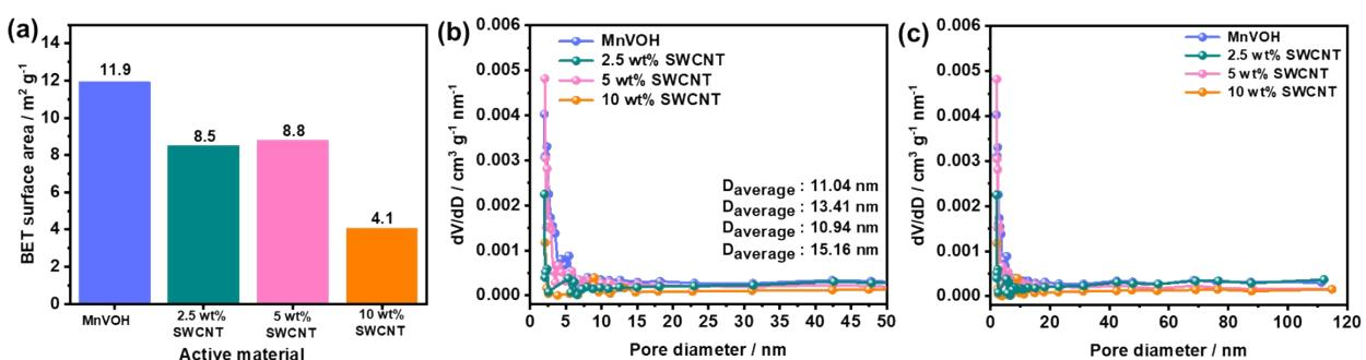
**Figure S3.** (a) Surface area, (b) pore size distribution curves, and (c) pore size distribution smaller than mesopores for MnVOH, 2.5 wt% SWCNT, 5 wt% SWCNT, and 10 wt% SWCNT.
