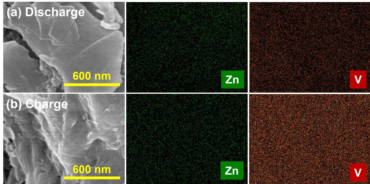
**Figure S16.** SEM images and the corresponding EDS mapping images of fully discharged (a) and charged (b) electrode materials of MnVOH@SWCNT (5 wt% SWCNT).
