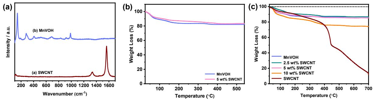
**Figure S4.** (a) Raman spectrum of SWCNT and MnVOH. (b) TGA curves collected over a temperature range of 25–550 °C for MnVOH and 5 wt% SWCNT in Ar atmosphere. (c) TGA curves collected over a temperature range of 25–700 °C for SWCNT, MnVOH, 2.5 wt% SWCNT, 5 wt% SWCNT, and 10 wt% SWCNT in air atmosphere.
