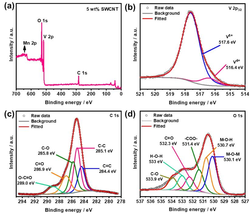
**Figure S6.** XPS wide spectrum of 5 wt% SWCNT: (a) Survey, (b) V 2p<sub>3/2</sub>, and (c) C 1s and (d) O 1s.
