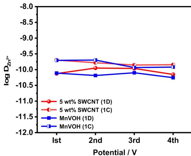
**Figure S12.** Comparison of the diffusion coefficient of the 5 wt% SWCNT and MnVOH electrodes measured using EIS method.
