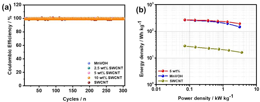
**Figure S10.** (a) Coulombic efficiency vs. cycles for MnVOH, 2.5 wt% SWCNT, 5 wt% SWCNT, and 10 wt% SWCNT. (b) Ragone plots of SWCNT, MnVOH, and 5 wt% SWCNT.
