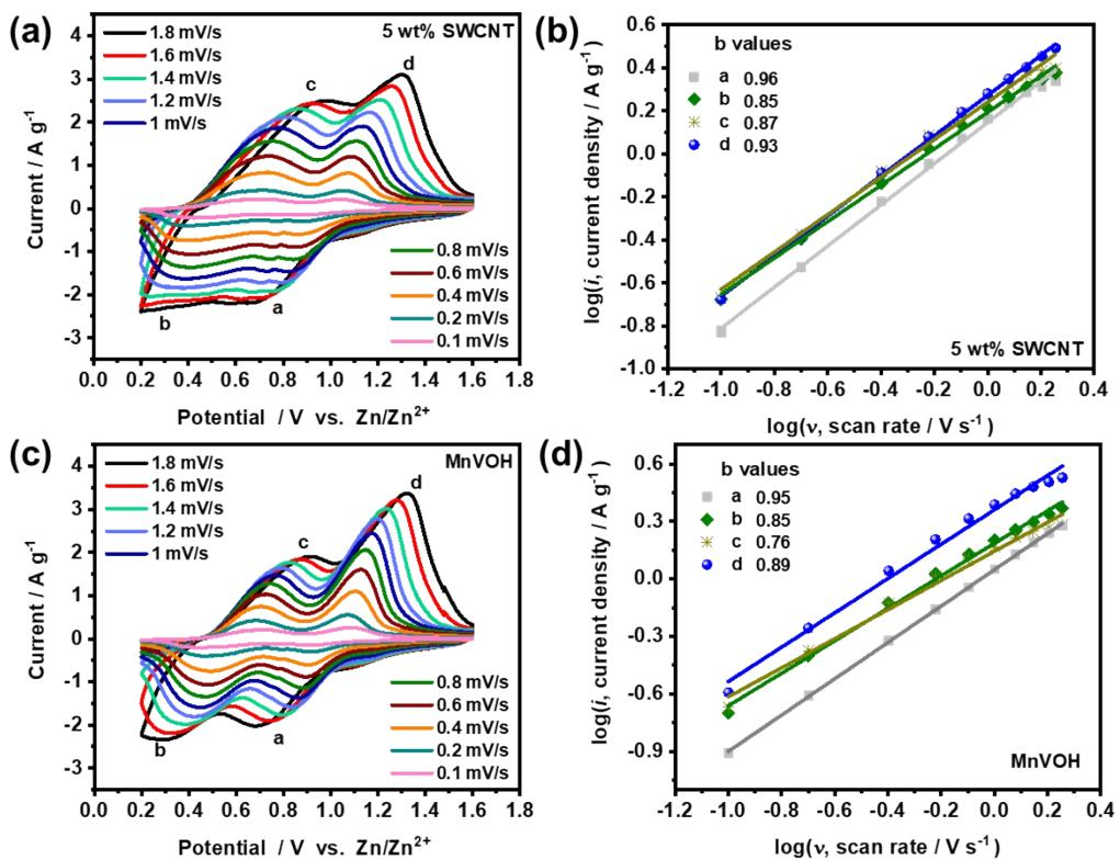
**Figure S9.** CV curves collected at different scan rates ( $0.1\text{--}1.8 \text{ mV s}^{-1}$ ) for (a) 5 wt% SWCNT , (c) MnVOH. Determination of the b-value at intercalation and deintercalation peaks of five peaks obtained in the CV curves for (b) 5 wt% SWCNT, (d) MnVOH.
