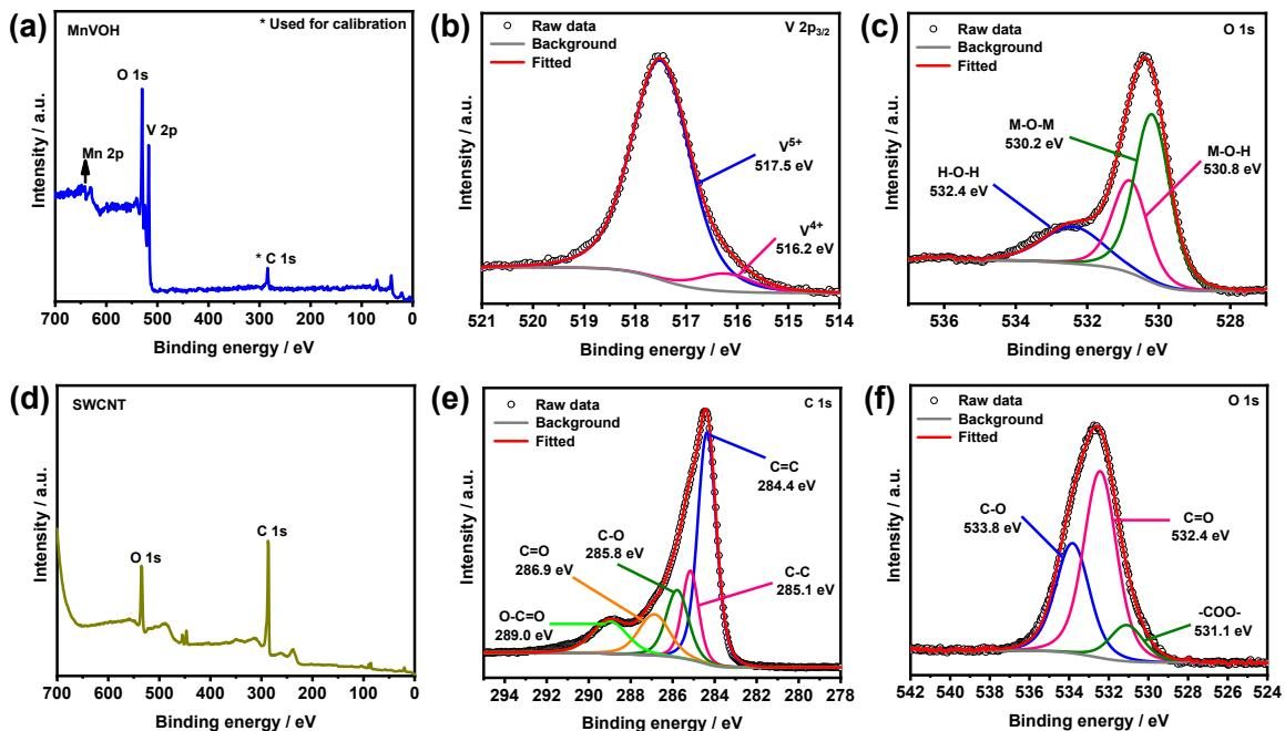
**Figure S7.** XPS spectrum of MnVOH: (a) Survey, (b) V 2p<sub>3/2</sub>, and (c) O 1s; XPS spectrum of SWCNT (d) Survey, (e) C 1s, and (f) O 1s.
