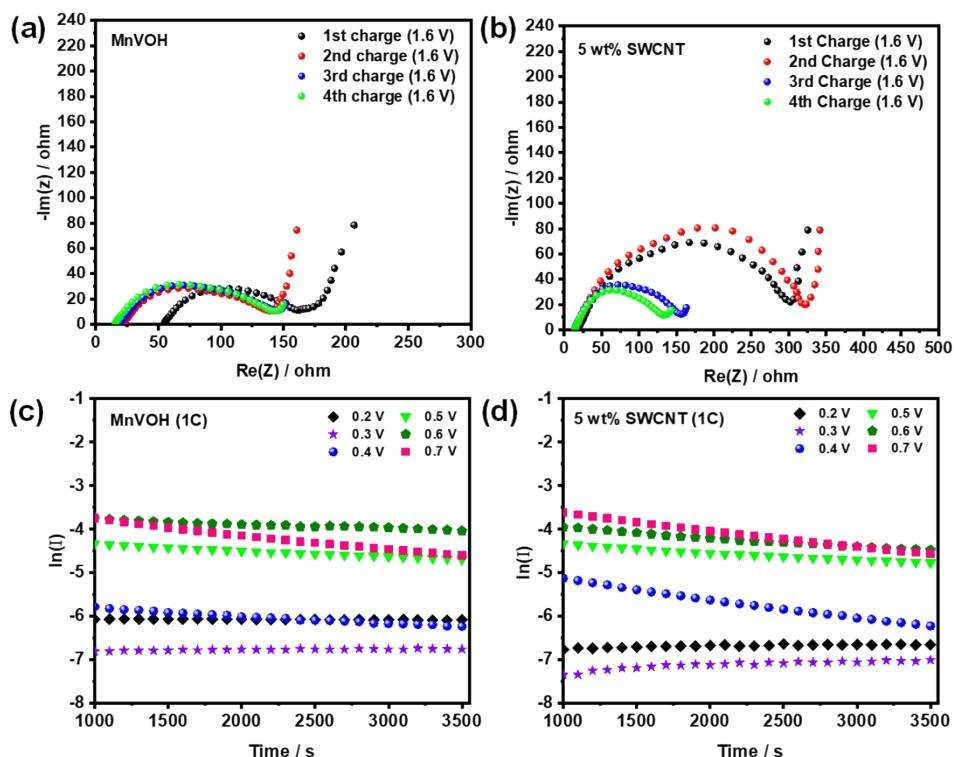
**Figure S11.** (a–b) Nyquist plots at fully charged state during 1st, 2nd, 3rd, and 4th cycles; (c–d)  $\ln(I)$  vs. time of chronoamperometry.
