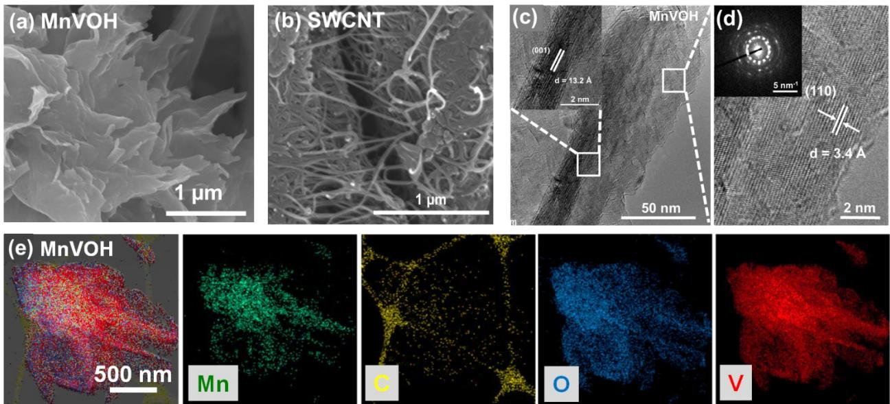
**Figure S1.** FESEM image of (a) MnVOH, and (b) SWCNT. HRTEM images of MnVOH with: (c) 13.2 Å interlayer spacing; (d) 3.4 Å interlayer spacing (inset is SAED pattern). (e) TEM-EDX mapping images of MnVOH.
