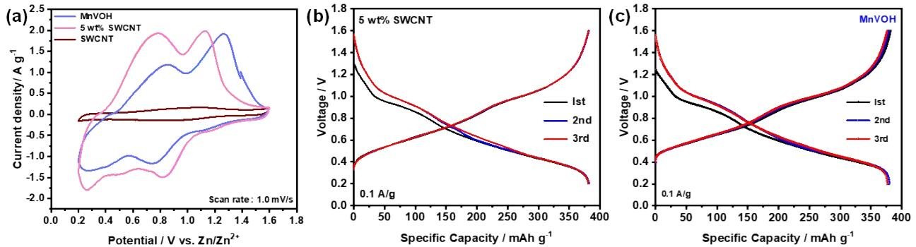
**Figure S8.** Electrochemical performance: (a) Cyclic voltammetry of MnVOH, 5 wt% SWCNT, and SWCNT at a scan rate of  $1.0 \text{ mV s}^{-1}$ . GCD curves of (b) 5 wt% SWCNT, and (c) MnVOH at a current density at  $0.1 \text{ A g}^{-1}$ .
