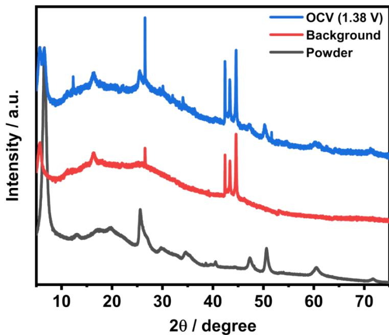
**Figure S15.** XRD patterns of pristine powder, background, and OCV for *operando* XRD measurement.
