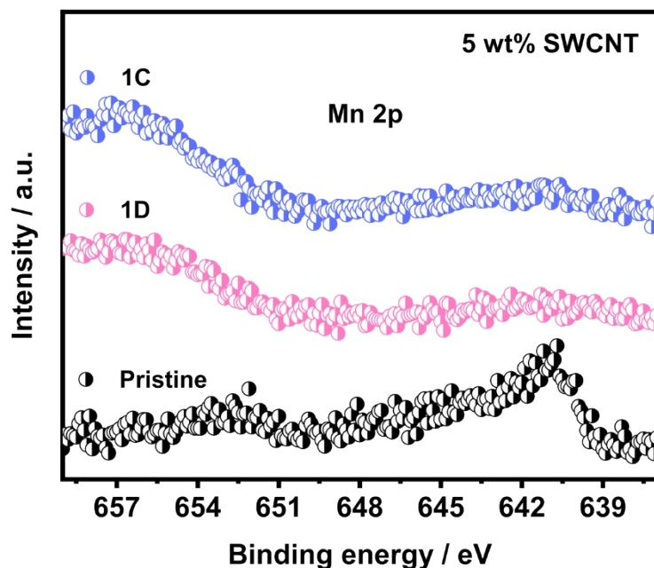
**Figure S14.** Ex-situ XPS of Mn 2p in the pristine, discharge to 0.2 V, and charge to 1.6 V states in the first cycle.
