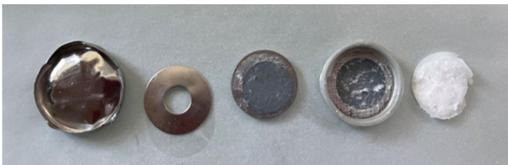
Figure S10. Photograph of the disassembled Zn/Zn cells after cycling in ZGN.
