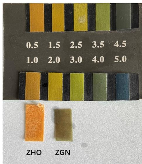
Figure S22. PH value of the ZHO and ZGN electrolytes.
