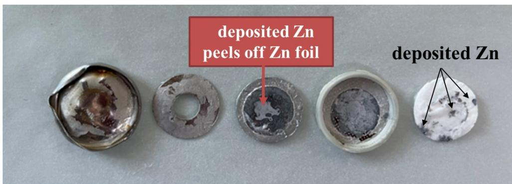
Figure S9. Photograph of the disassembled Zn/Zn cells after cycling in ZHO.
