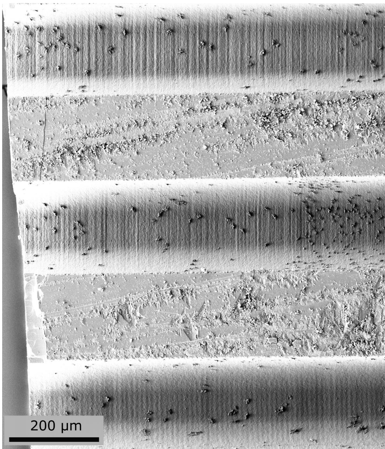
Figure S7. SEM image of grooves 7-9 (top to bottom) after 5 hours of exposure to CO 2 at 330°C, i.e. NaNO 3 -MgO_B 5 hours-CO2 . MgCO 3 particles grow close and far away from the TPB (top of groove). NaNO 3 has been removed by a rinse in water and the sample was coated by PtPd prior to SEM (secondary electron) imaging.
