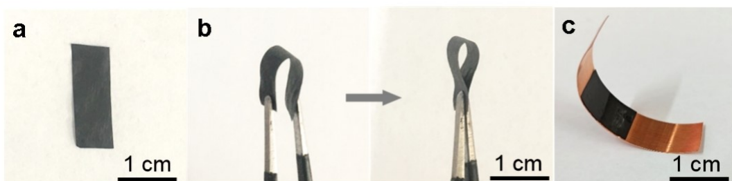
Fig. S9 (a) The optical photos of oblong SLMP films. (b) The SLMP films can be bent 180^\circ , and can be attached to a semicircular copper electrode in (c).
