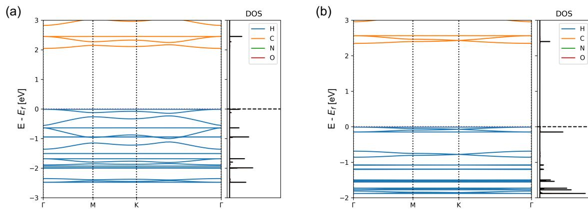
**Fig. S4.** Electronic band structures of monolayer Tp-Azo (a) and monolayer DAAQ-TFP (b).
