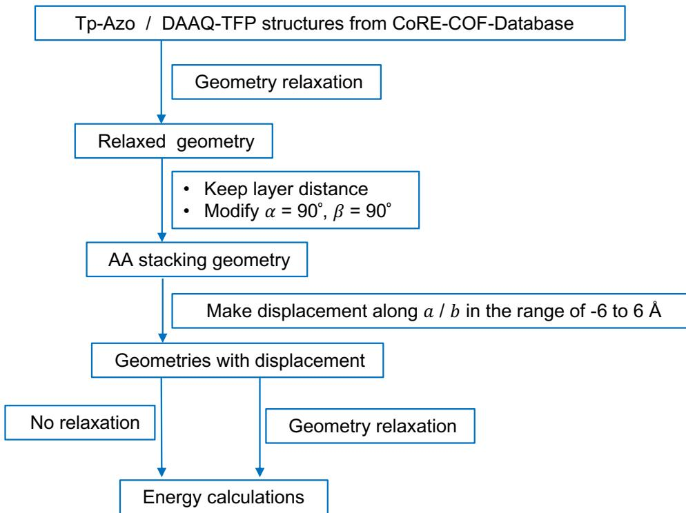
**Fig. S1.** Workflow of displacement process.
