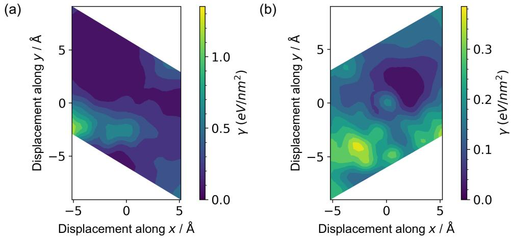
**Fig. S3.** Potential energy surfaces (PES) for rigid layer displacements along *a* and *b* sides of (a) Tp-Azo and (b) DAAQ-TFP. Note, the PES reported in the main text includes geometry relaxation.
