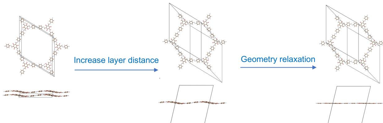
**Fig. S2.** Process of forming monolayer and the binding energy calculation of Tp-Azo COF. The upper figures are viewed looking down the  $c$  axis, and the lower figures are viewed along the  $ab$  plane. The layer distance in geometry relaxation keeps 30 Å.
