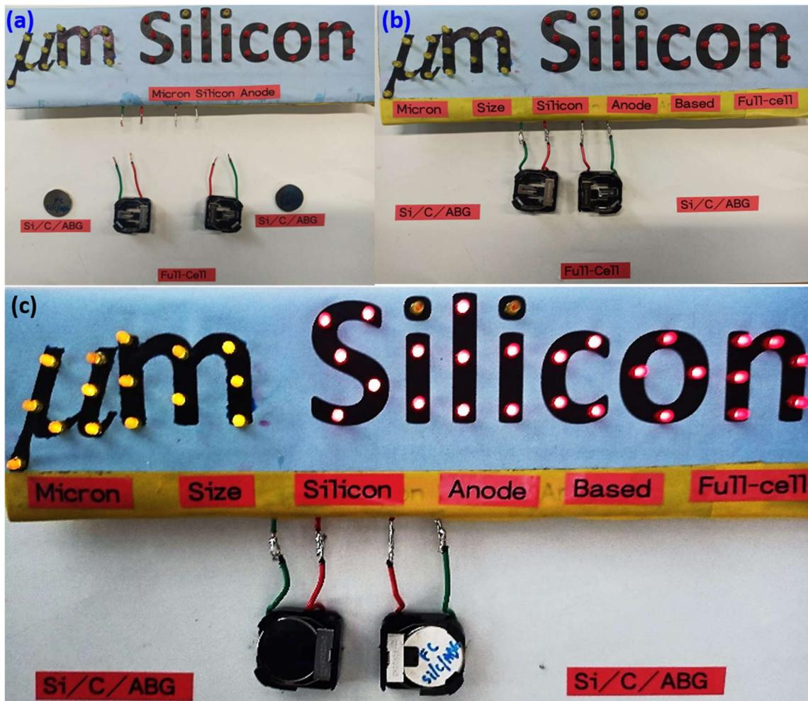
**Figure S14.** The optical photo graphs of (a,b) LED arrangement, cell holders and a pair of NCA (cathode) // Si/C/ABG (anode) based full-cells. (c) Powering the LED arrangement using NCA // Si/C/ABG based full-cells.
