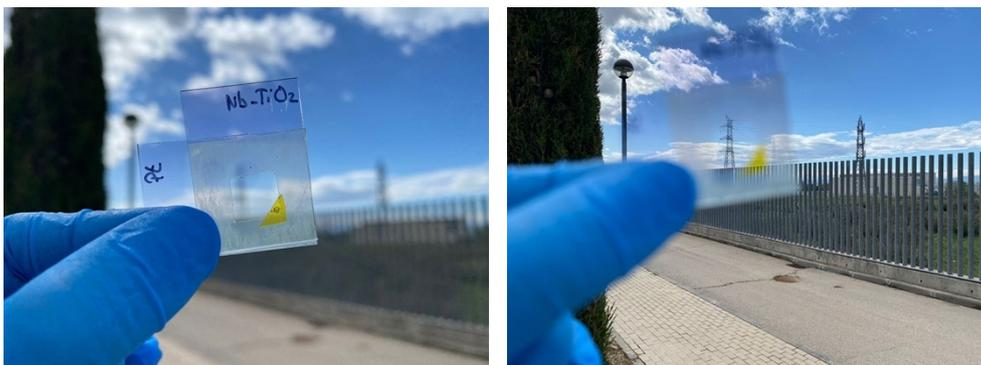
Figure S19. Images of the smart window lab scale device with high optical transparency.
