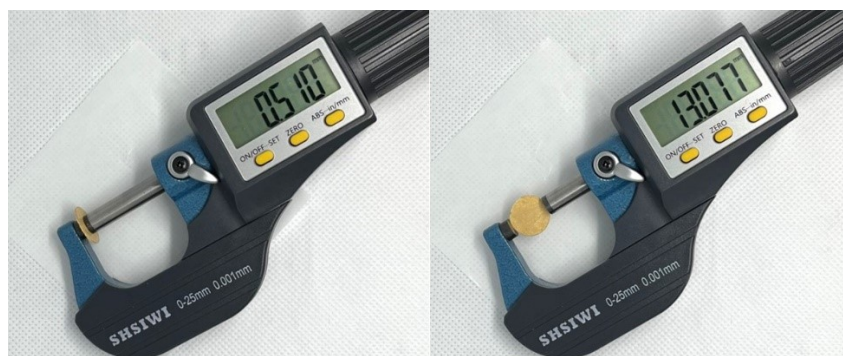
Figure S11. The S-PD pellet was obtained by the classic powder's pressing method (18 MPa).
