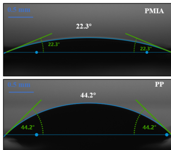
Fig. S9. Contact angle images of the PP and PMIA separators.
