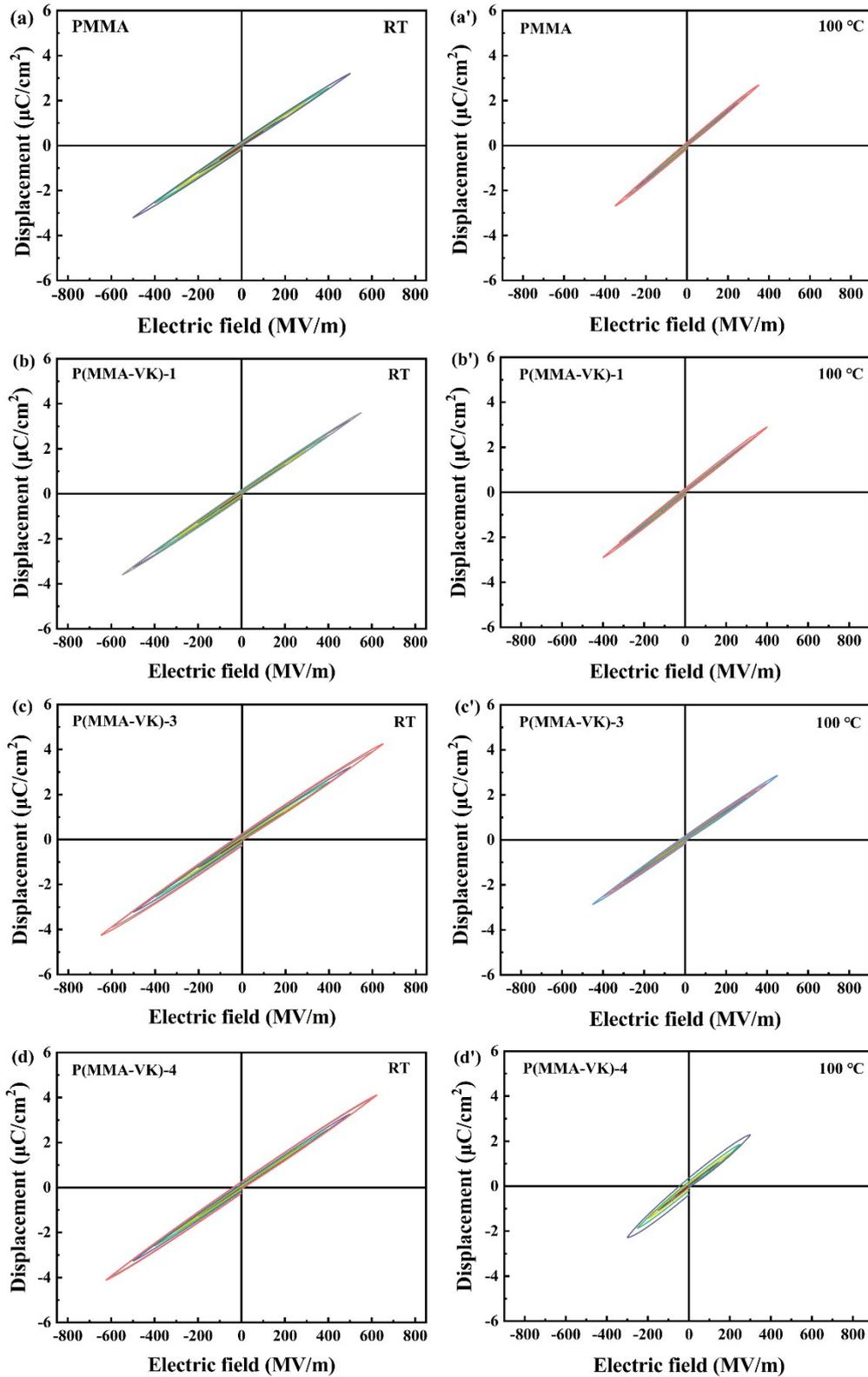
**Figure S4.** Bipolar  $D$ - $E$  loops at room temperature for (a) PMMA, (b) P(MMA-VK)-1, (c) P(MMA-VK)-3, (d) P(MMA-VK)-4, and at 100°C for (a') PMMA, (b') P(MMA-VK)-1, (c') P(MMA-VK)-3, (d') P(MMA-VK)-4.
