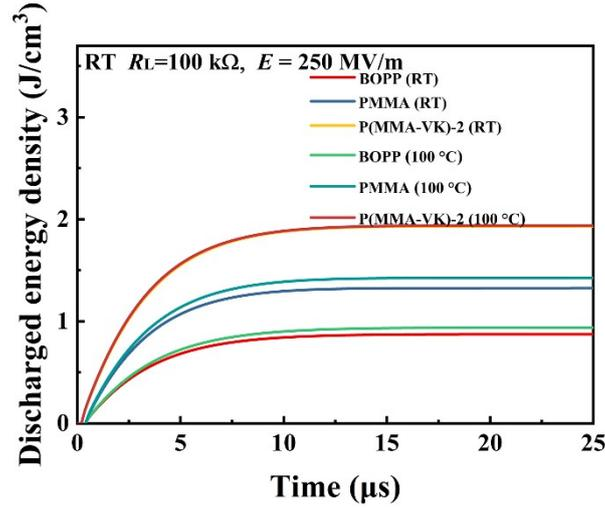
**Figure S7.** Discharged energy density of the prepared polymer and commercial BOPP.
