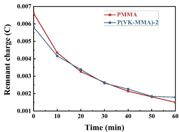
**Figure S11.** The remnant charge over time after removing the applied field for PMMA and P(MMA-VK)-2.
