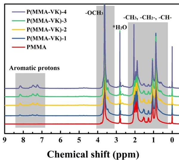
**Figure S1.** <sup>1</sup>H NMR spectra of the prepared polymers.
