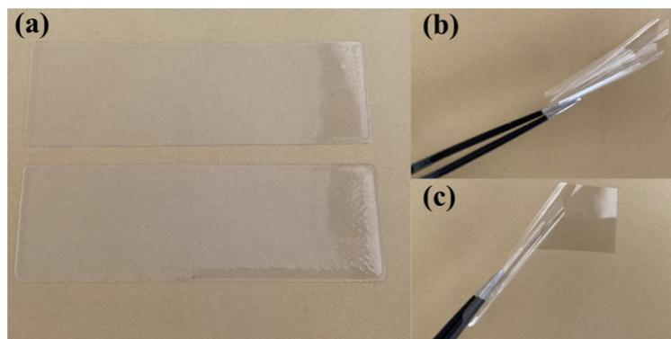
**Figure S9.** (a) Digital image of P(MMA-VK)-2 film with a thickness of 12  $\mu\text{m}$  and its digital images after (b) wrapping and (c) folding.
