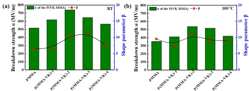
**Figure S8.** Breakdown strength  $\alpha$  and shape parameter  $\beta$  of the prepared polymers at ambient temperature and 100°C.
