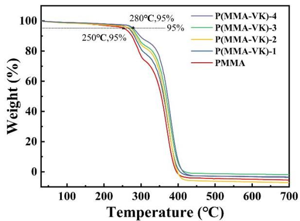
Figure S3. TGA traces of the prepared polymers.
