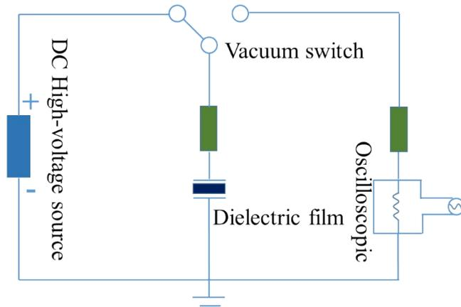
**Figure S6.** Schematic circuit of the discharge experiment.
