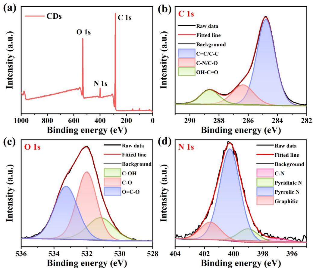
**Fig. S2.** (a) XPS survey spectra of CDs. High-resolution XPS spectra of (b) C 1s and (c) O 1s and (d) N 1s of CDs.
