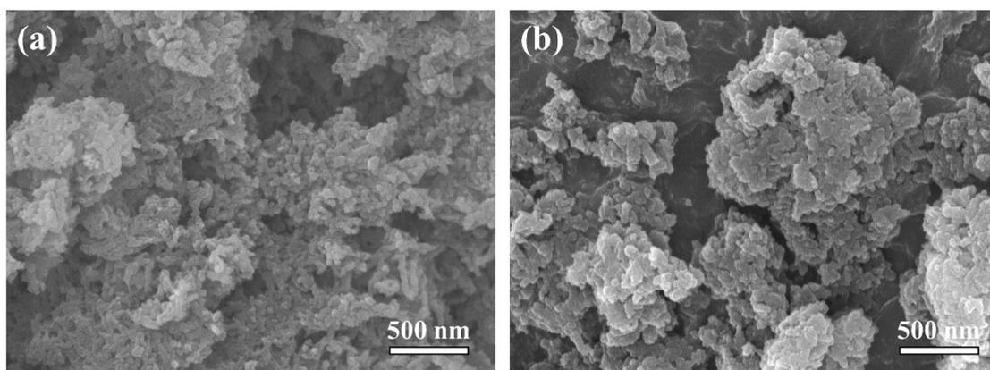
**Fig. S3.** SEM images of (a) COF and (b) COF@CDs.
