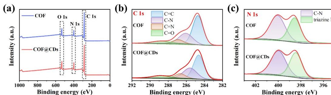
**Fig. S1.** (a) XPS survey spectra of COF and COF@CDs. High-resolution XPS spectra of (b) C 1s and (c) N 1s of COF and COF@CDs.
