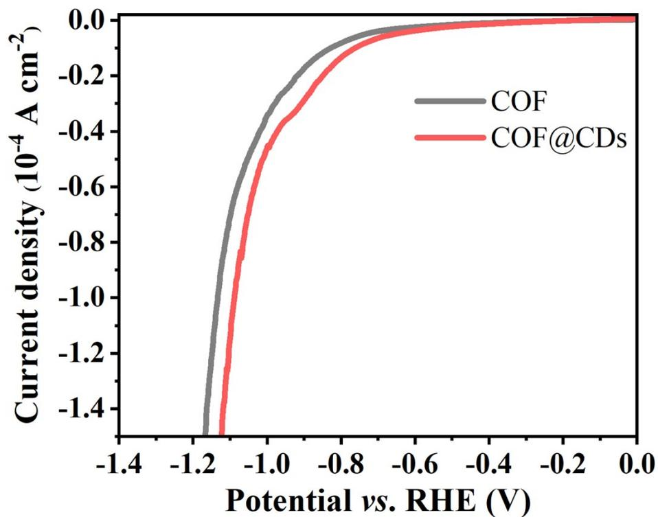
Fig. S5. Polarization curves of COF and COF@CDs.
