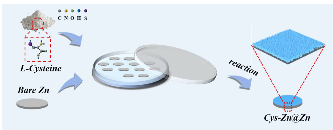
Figure S1. Schematic illustration of fabricating ultrathin L-cysteine complex layers on the Zn foil (Cys-Zn@Zn).
