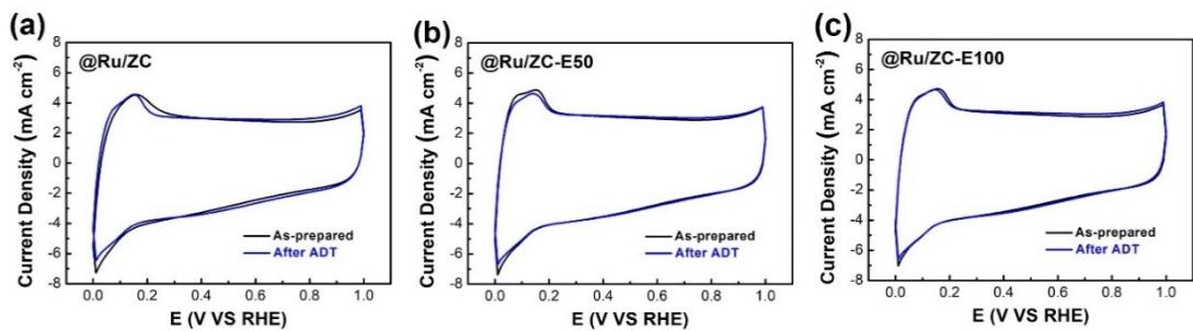
**Figure S6.** CV curves before and after ADT for Ru/ZC, Ru/ZC-E50, and Ru/ZC-E100.
