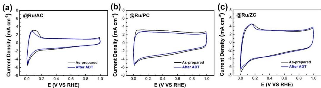
**Figure S3. CV curves before and after ADT for Ru/AC, Ru/PC, and Ru/ZC.**
