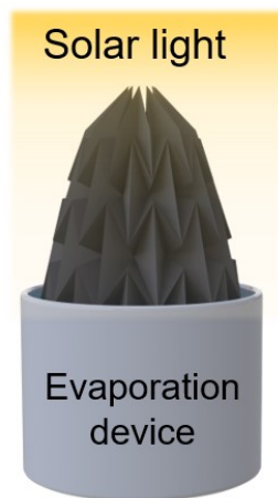
Fig. S7. Schematically showing the solar light provided by the solar simulator shines vertically on the evaporation device in the indoor evaporation test.
