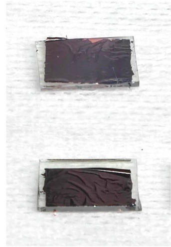
Figure S16. (a) Samples with the architecture of ITO/PTAA or AlCl 4 -PTAA/Perovskite/Cu immersed in chlorobenzene solvent. The integrated perovskite/metal films had been detached from the substrates. The size of the substrate was reduced to 6 mm × 9 mm. One reason is to reduce the soaking time. Another reason is to ensure that the perovskite thin film of the PTAA sample was fully covered. (b) Prepared samples with the bottom sides up for the measurements on buried interfaces.
