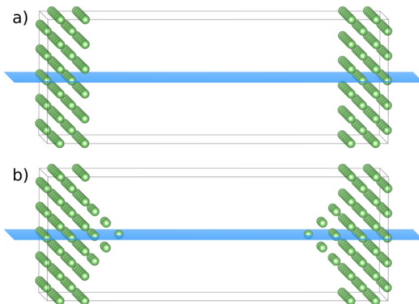
Fig. S7: Simulation cell a) without and b) with a lithium tip. The electrostatic potential profiles provided in the main manuscript are projected in the [200] plane, as represented by the blue planes.
