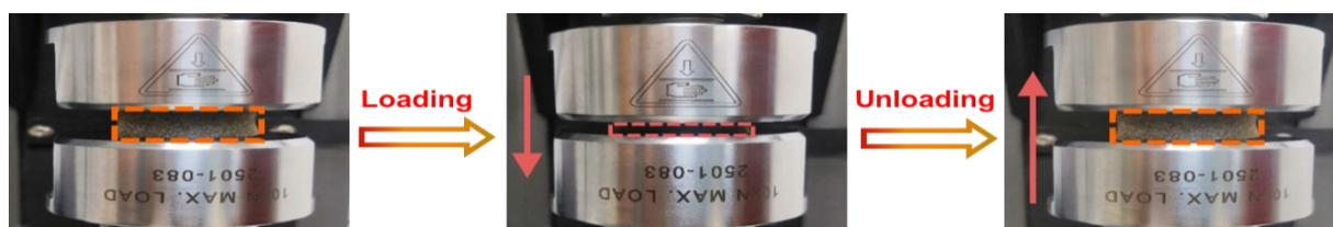
**Figure S15.** Compression recovery of the PSiNFs@PU sponge at 60 % compression strain.
