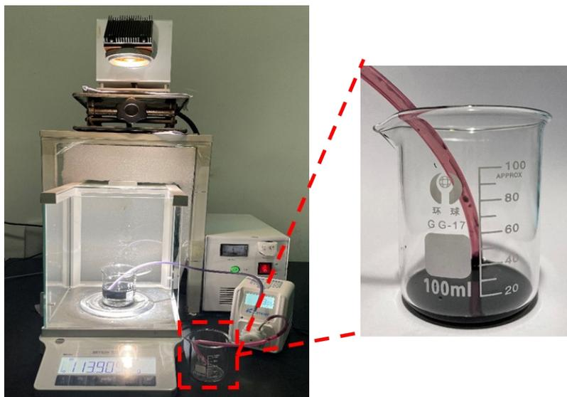
**Figure S20.** Photograph of continuous oil absorption of the PSiNFs@PU sponge under light condition (power density: 1.00 kW /m<sup>2</sup>). The tests were conducted at an environmental temperature of 25 °C.
