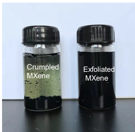
Figure S1 The digital photo of exfoliated few-layered MXene solution and crumpled MXene flocculation.
