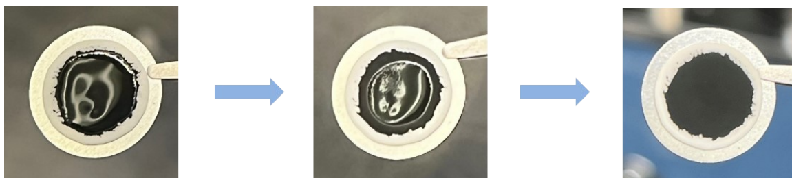
Figure S2. Cathode appearance evolution during 7 min drying process.
