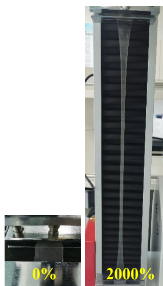
Figure S6. Optical photographs of TSPU elastomer at 0% (left) and 2000% (right) strains.
