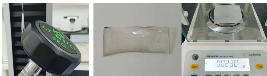
Figure S8. The weights of dumbbell and TSPU sample used to lift up dumbbell.
