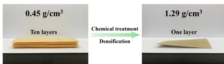
Fig. S5 Digital photos of CCNB 0 made from ten layers of basswood veneers.
