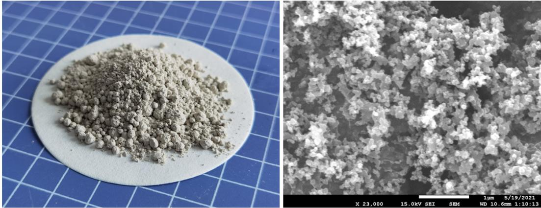
**Figure S3.** Digital photo and SEM image of  $n\text{-Si}_3\text{N}_4$  powder.
