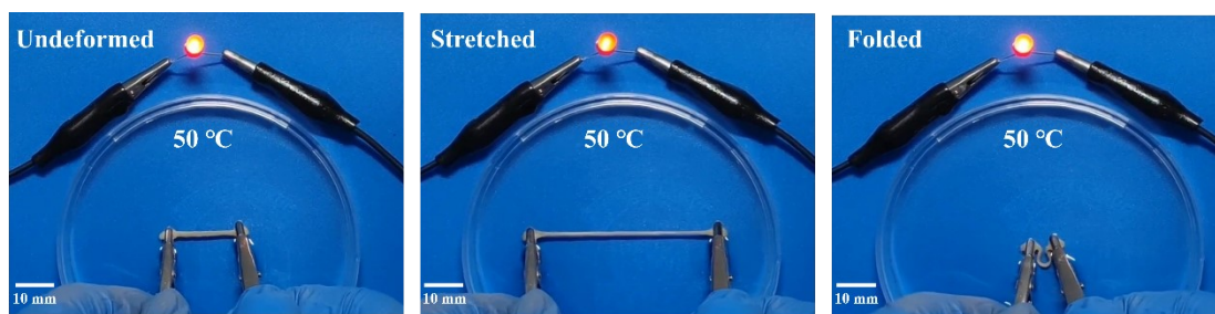
Fig. S14. Mechanical response of hydrogels under thermal stimulation. Brightness changes of LED in the undeformed, stretched and folded states of \text{Ag}_{0.3} -PNIPAM hydrogels in 50 °C water.
