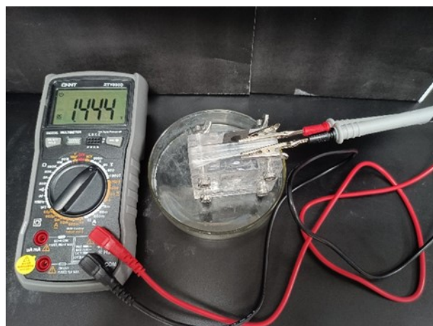
Fig. S23 The photo of open-circuit voltage measurement (with a multimeter) for CoSA@NPC-based ZAB.
