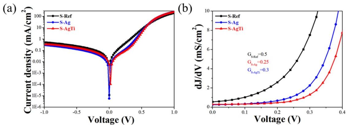
**Figure S5.** (a) Dark  $J$ - $V$  curves, and (b) Shunt conductance  $G$  characterizations of S-Ref, S-Ag and S-AgTi devices.
