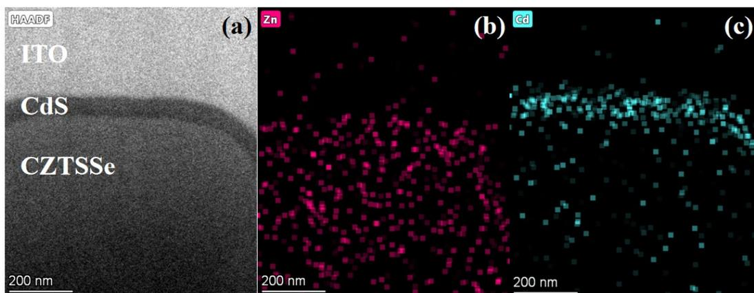
**Figure S6.** TEM image and TEM-coupled element mapping results for the champion S-AgTi device: (a) Cross-sectional TEM image, (b) Zn, and (c) Cd elemental mapping images.
