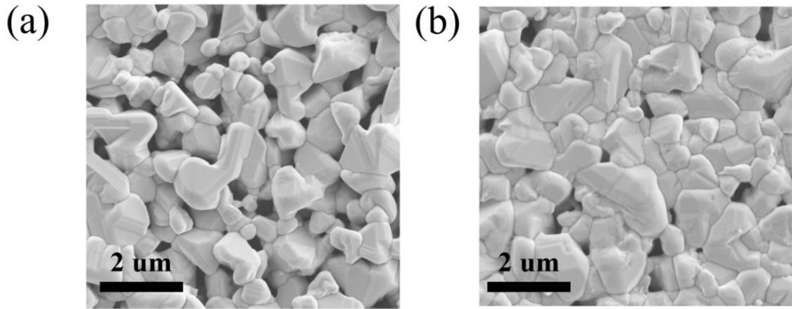
**Figure S2.** SEM images of (a) Pristine, and (b) Ti substituted CZTSSe thin films.
