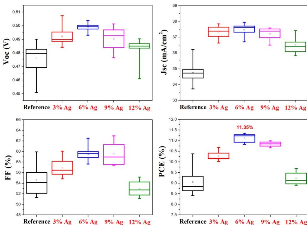
**Figure S1.** The statistic photovoltaic performances ( $V_{OC}$ ,  $J_{SC}$ , FF and PCE) of CZTSSe-based solar cells with various Ag substitution concentration.
