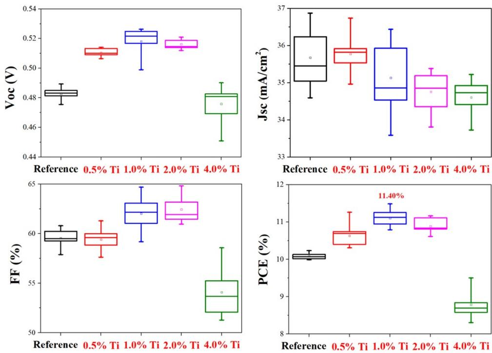
**Figure S3.** The statistic photovoltaic performances ( $V_{OC}$ ,  $J_{SC}$ , FF and PCE) of CZTSSe-based solar cells with various Ti substitution concentration.
