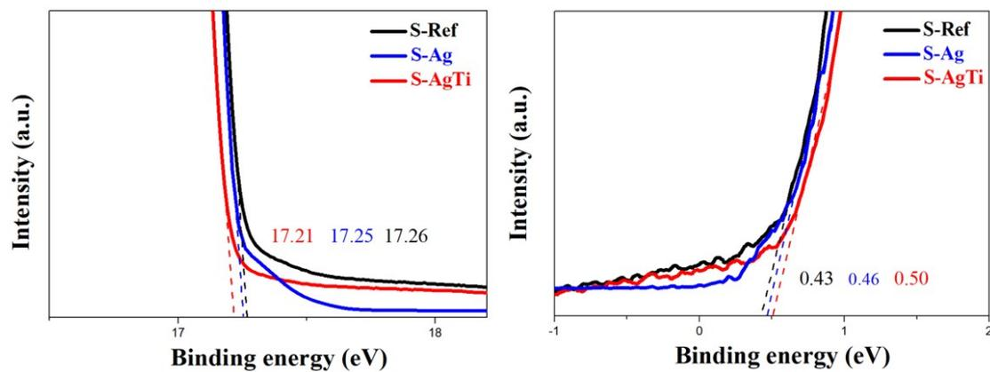
**Figure S8.** UPS characterizations: secondary electron cut-off (SEC) edge and valence band (VB) position of S-Ref, S-Ag and S-AgTi thin films.
