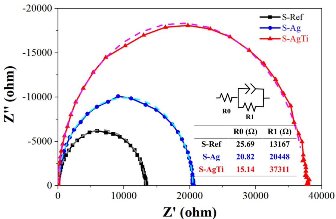
**Figure S7.** EIS Nyquist plots of S-Ref, S-Ag, and S-AgTi devices. Inset is the equivalent circuit and the corresponding parameters.
