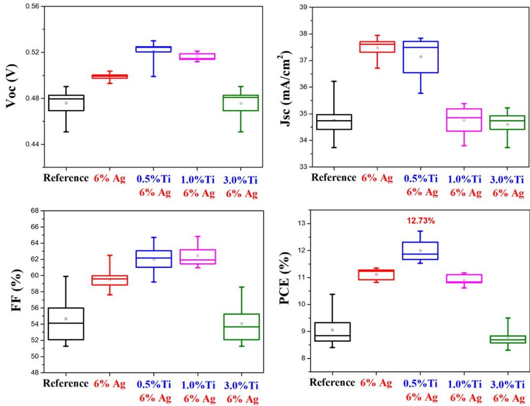
**Figure S4.** The statistic photovoltaic performances ( $V_{OC}$ ,  $J_{SC}$ , FF and PCE) of 6%-Ag-substituted CZTSSe solar cells and various Ti substitution concentration.
